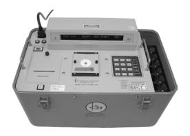
Two configurations of the Model 3605-A Thermo Unit are available. Part No. 3605A-1-1 includes four adapter chucks in the following bore diameters: 1/4", 3/8", 7/16", and 9/16". Part No. 3605A-1-101 includes 12 adapter chucks conforming to specific U.S. Navy requirements. Compartments in the carrying case permit up to a dozen adapter chucks to be stored and transported with the instrument.
