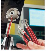
**Fig 22.** Testing strength of crimped connections using HT20 grips
