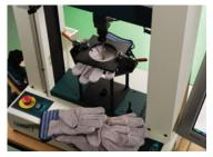
**Fig 30.** Testing the puncture resistance of work gloves
