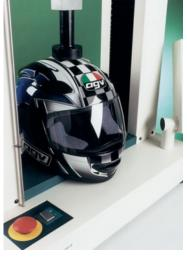
Fig 27. Compression test on crash helmet
