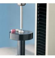
Fig 15. Testing the crushing strength of pills
