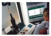
Fig 31. Testing the extraction forces of new material for wine bottle corks
