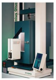
**Fig 26.** Model H10kS shown with an environmental chamber for testing at elevated or reduced temperatures; note the use of a laser extensometer that can be used with the chamber to determine the elongation of the sample
