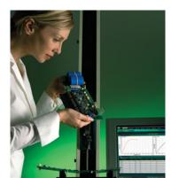
**Fig 8.** Model H1kS being used to find the tensile strength of a baby's pacifier
