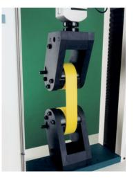
**Fig 28.** Testing webbing material using S453 grips
