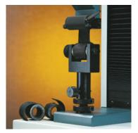
**Fig 17.** Checking the peeling strength of the outer layer of rubber hose, using a combination of standard and custom grips
