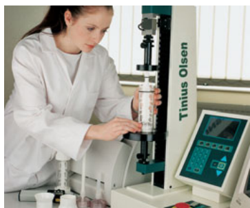
Fig 16. Testing the compressive resistance of a polymer cement mixer
