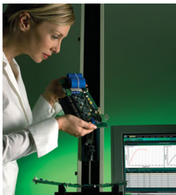
Fig 6. Testing of rigid plastics and use of Model 100R multi gauge length extensometer
