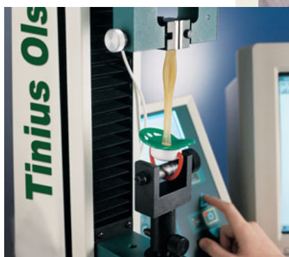
Fig 8. Model H1kS being used to find the tensile strength of a baby's pacifier
