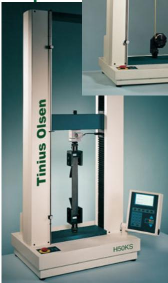
Fig 34. Model H50kS with model HT43 bollard grips testing seatbelt webbing
