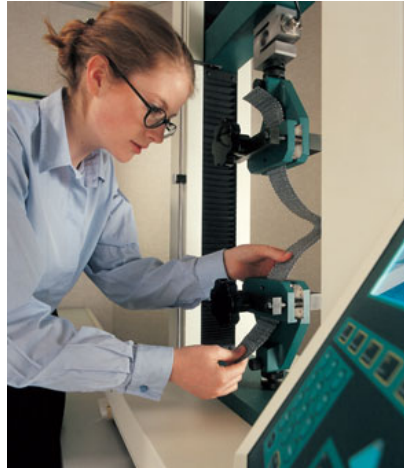
Fig 38. Machine being used to determine the strength of a flexible geo material
