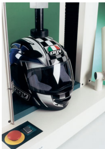
Fig 27. Compression test on crash helmet
