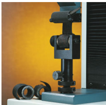
Fig 17. Checking the peeling strength of the outer layer of rubber hose, using a combination of standard and custom grips
