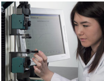
Fig 6. Testing of rigid plastics and use of Model 100R multi gauge length extensometer
