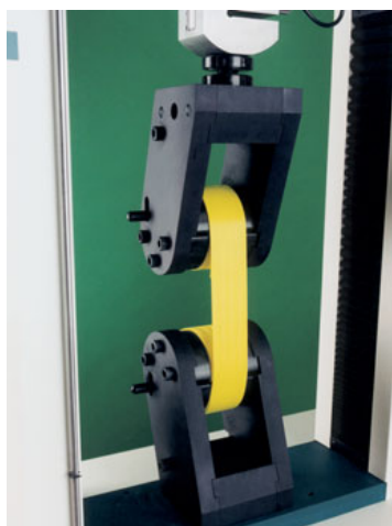
Fig 28. Testing webbing material using S453 grips
