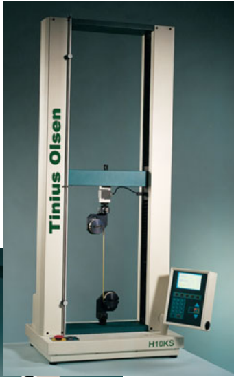
Fig 33. Model H10kS using split bollard grips to test PP and PE packing tapes
