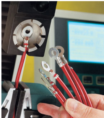
Fig 22. Testing strength of crimped connections using HT20 grips
