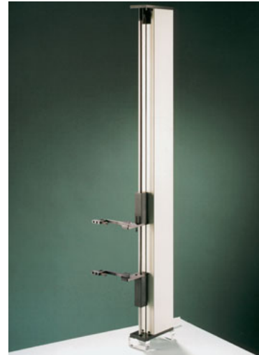
Fig 29. Tinius Olsen high travel extensometer, model 100RC
