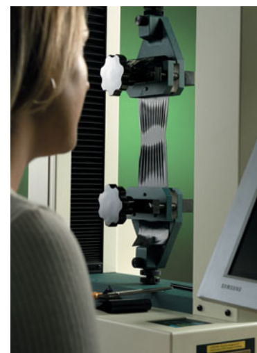
Fig 32. Tear test on rubber specimens
