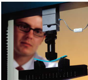
Fig 24. A 3 point bend test being performed with model HF72 flexural jig on plastic sample
