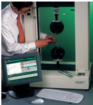
Fig 23. Dumbbell sample of sheet metal being tested with HW21 grips
