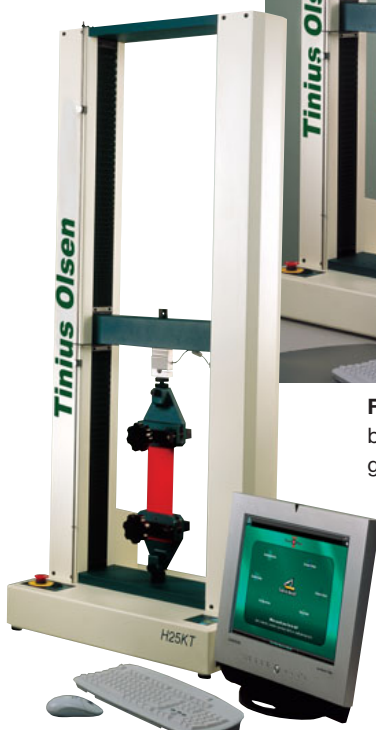
Fig 34. Model H50kS with model HT43 bollard grips testing seatbelt webbing
