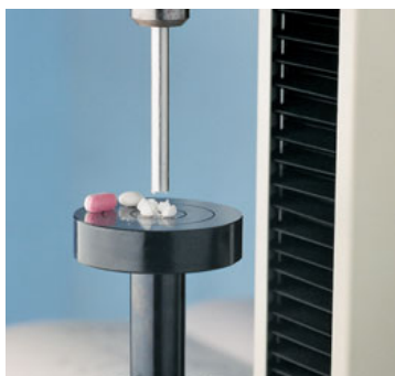
Fig 15. Testing the crushing strength of pills
