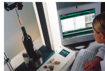
Fig 31. Testing the extraction forces of new material for wine bottle corks
