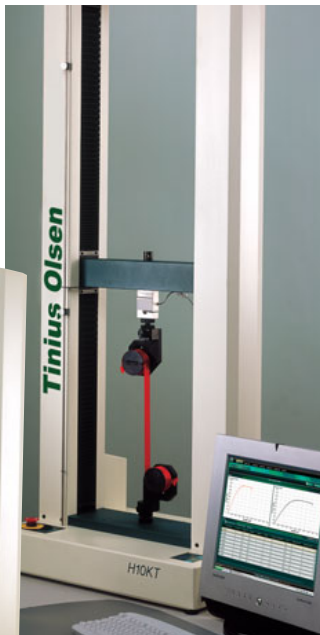
Fig 35. Model H10kT being used with HT29 grips to test thin rope
