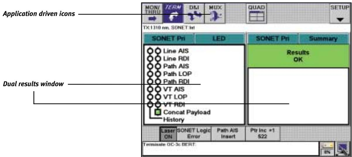
**Auto Configuration**—Support for auto configuration is provided in all key applications on the 2310. One-button touch configures different test parameters, such as framing, pattern, and tributary scan, and enables users to reduce the test set-up time required.
