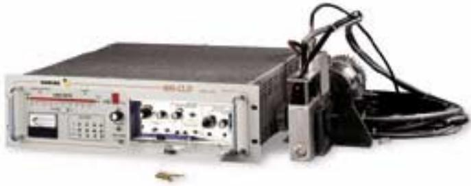
The Varian 990CLD Component Leak Detector is a modular leak-testing package that can be integrated into virtually any testing system. The electronics module of the 990 can be separated from the sensing module and vacuum pumps by as much as 15-feet, permitting a high degree of flexibility in your system design.
