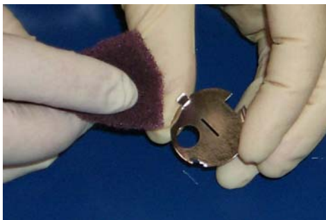
Figure 4-20 Discolored Ground Slit Plate
