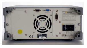
The V60 Series rear panel layout includes three standard remote interfaces: A fully programmable RS232 port, a PLC Interface port and a High Voltage Scanner control port. Available options include GPIB and rear terminal outputs.
