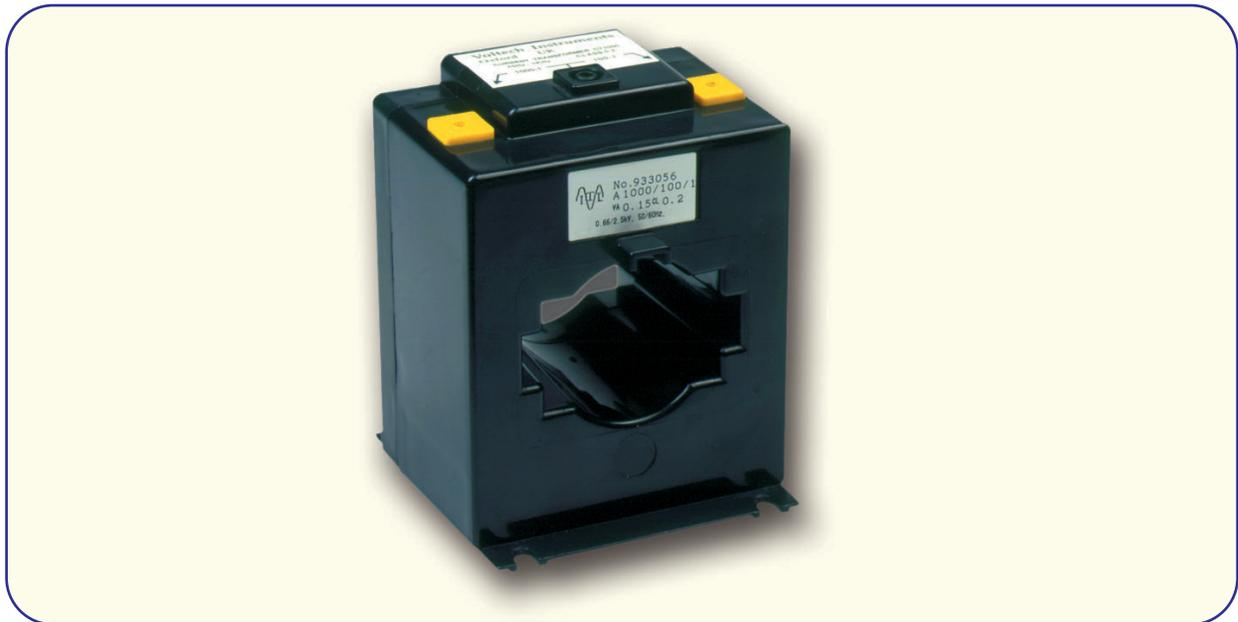
The Voltech CT1000 is a toroidally wound AC current transformer that extends the range of Voltech power analyzers such as the PM100, PM300 or PM3000A to 1200A rms. Close-tolerance current ratios provide a measurement accuracy of better than 0.2%, making the CT1000 suitable for precision-grade measurements.
