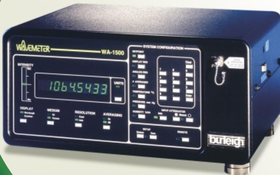
The WA-1500 WAVEMETER® Laser Wavelength Meter measures the absolute wavelength of virtually any CW laser to the highest accuracy available,  $\pm 0.2$  ppm ( $\pm 0.0002$  nm at 1000 nm). When the highest accuracy is not required, the WA-1000 is available as a lower cost alternative to provide an absolute wavelength accuracy of  $\pm 1.0$  ppm ( $\pm 0.001$  nm at 1000 nm).
