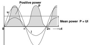
When the phase difference between the voltage and current is  $\boldsymbol{\varphi}$
