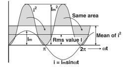
The rms value (effective value) is the value of the DC signal that generates the same heating effect as the AC signal. If the value of the DC signal that generates the same heating effect is expressed as I, then
