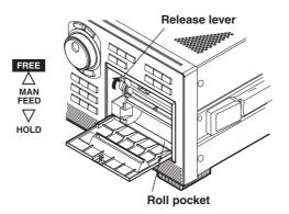
3. With approximately 13 cm of the **roll paper** unrolled, place the roll paper in the roll pocket in the direction indicated by the figure below.
