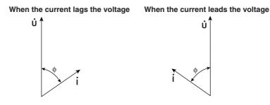
The vector display of the voltage and current of a three-phase AC signal would look something like the following figure.
