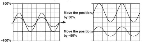
• When the zoom factor is not 1, the value equal to the measurement range × 3 (100%) or measurement range × 6 (100%) when the crest factor is set to 3 or 6, respectively, is not located at the upper and lower limits of the screen as shown in the following figure. Set the position by paying attention to the zoom factor. The following figure shows an example when the crest factor is set to 3.
