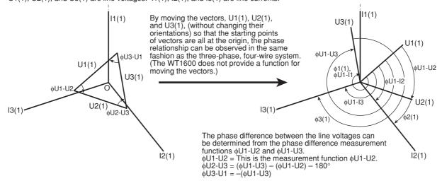
**Vector display when the wiring system is 3P3W (three-phase, three-wire)** U1(1), U2(1), and U3(1) are line voltages. 11(1), 12(1), and I3(1) are line currents. However, U3(1) and I3(1) are not actually measured for the three-phase, three-wire system. The vectors are displayed through computation.
