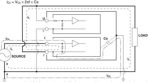
When measuring high frequencies as in this instrument, this error,  $i_{Cs}$ , cannot be ignored. By connecting the current input terminal of the instrument to the side that is close to the earth potential of the power source (SOURCE), the terminal of the current measurement circuit of the instrument approaches the earth potential. Thus,  $V_{Cs}$  becomes approximately zero and very little  $i_{Cs}$  flows.
