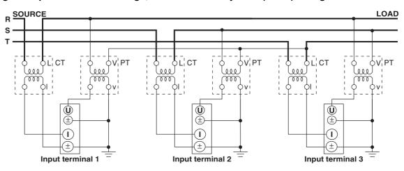
Wiring Example of a Three-Phase, Four-Wire System (3P4W) Using PT and CT
