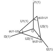
• By moving the vectors, U1(1), U2(1), and U3(1), so that the starting points of vectors are all at the origin, the phase relationship can be observed in the same fashion as the three-phase four-wire system. For the relationship between the positions of the vectors after moving them, see "Vector Display of Harmonics" in section 1.8. (The WT1600 does not provide a function for moving the vectors.)
