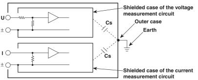
For example, we will consider the case when one side of the power source and the outer case are grounded.
