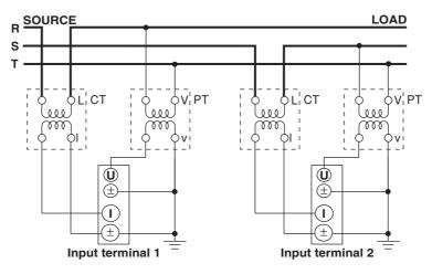
Wiring Example of a Three-Voltage, Three-Current System (3V3A) Using PT and CT
