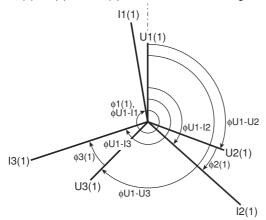
Vector display when the wiring system is 3P4W (three-phase, four-wire)
