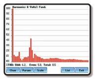
can cause small, almost imperceptible variations in performance that aggregate to effect significant long-term damage. Current harmonics generated by a source can pollute the entire power system without being affected itself. The PowerXplorer captures detailed harmonics, interharmonics and subharmonics to effectively trouble shoot the complex problems caused by these events.
