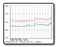
impedances, which causes voltage distortion as well. This distortion can have a significant derating effect on equipment such as motors and transformers, causing overheating that shorten equipment life. The PowerXplorer measures the full range of arithmetic, vector and sequencing parameters contained in IEEE 1459, to evaluate distortion and restore balanced loads.
