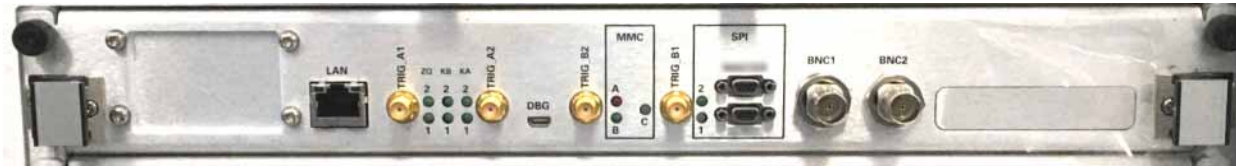
Figure 4-7 UXM 5G Rear Panel -- DCB+ Connectors
