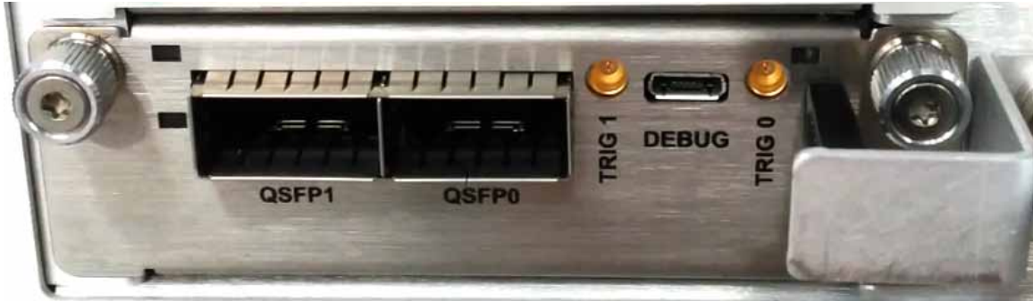
Figure 4-4 UXM 5G Rear Panel -- E7515B-FP1 card connectors
