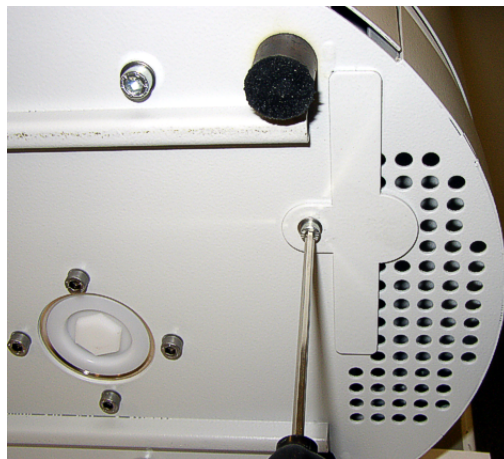
Fig. 3: Loosening the air filter cover
