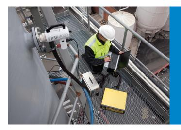
DX4000 is the world's smallest FTIR emissions monitoring system.
