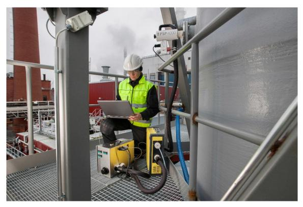
Gasmet FTIR gas analyzers have been used for high-quality emission-related research already for more than a decade. Gasmet analyzers have been used to measure pollutants and greenhouse gases from e.g. waste incinerators and wastewater treatment plants as well as for catalyst research.
