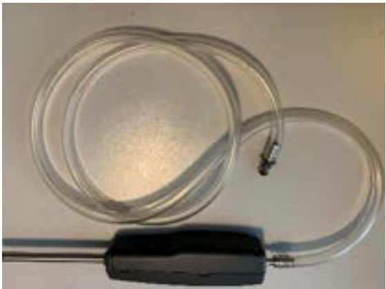
Gaset Sample Probe with 1. Teflon Tubing (white) recommended for sampling 2. Tygon tubing (Clear) recommended for background measurement
