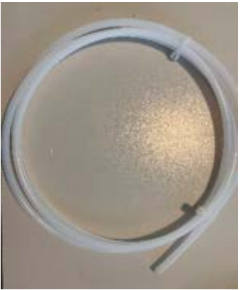
Gaset Sample Probe with 1. Teflon Tubing (white) recommended for sampling 2. Tygon tubing (Clear) recommended for background measurement
