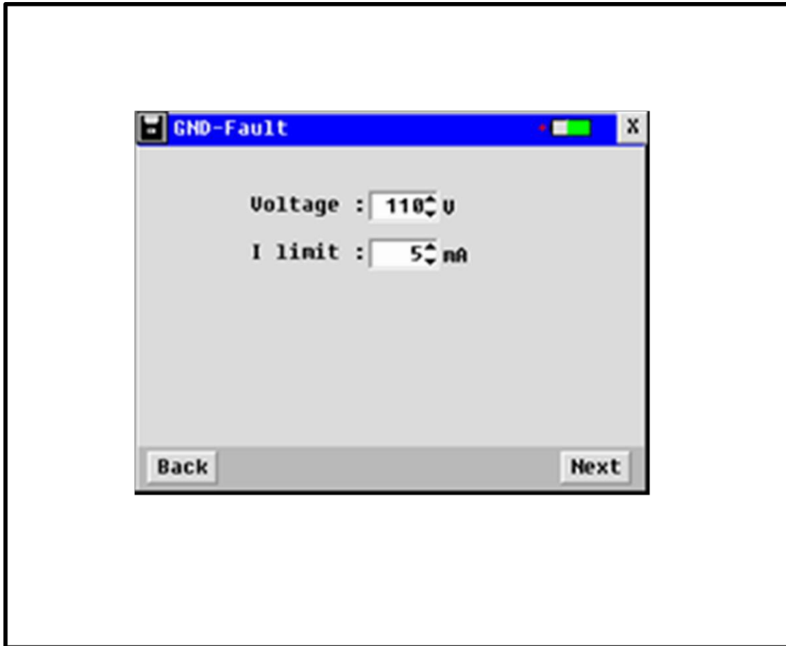
Figure 4-4 Voltage and Current Limit Settings
