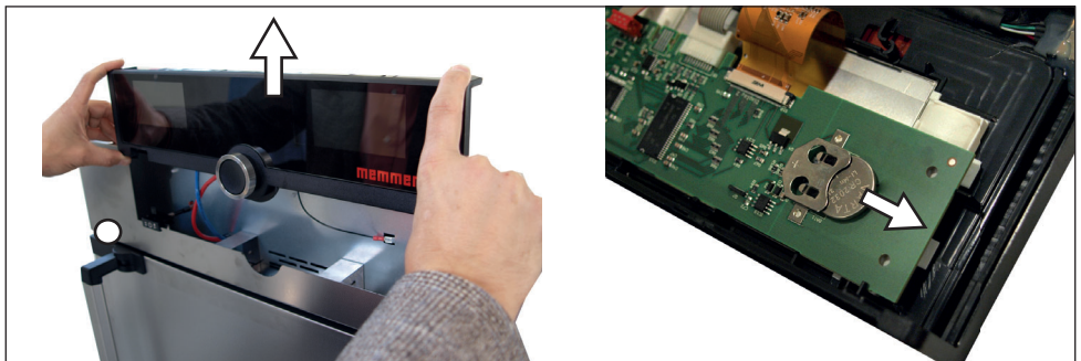
Fig. 25 Removing the lithium battery
