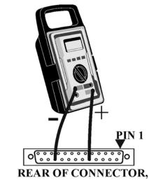
CONNECT PINS 18 AND 23 FOR 4-20 mA OUTPUT. JUMPER IS SET TO 'I' or 2&3 Figure 2
