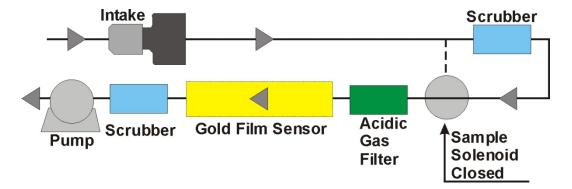
After 2 seconds, the sample solenoid bypass opens, closing off the scrubber filter from the flow system.
