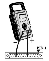
REAR OF CONNECTOR, CONNECT PINS 18 AND 23 FOR 0-2 VOLT OUTPUT. JUMPER IS SET TO 'V' or 1&2 Figure 1
