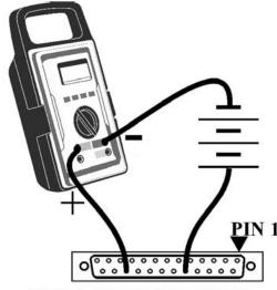
REAR OF CONNECTOR, CONNECT PINS 18 AND 23 FOR 4-20 mA OUTPUT. JUMPER IS SET TO 'I' or 2&3 Figure 3
