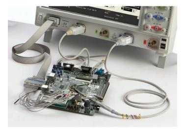
Designing with Xilinx FPGAs? Use the FPGA dynamic probe for rapid internal FPGA measurements. Using I<sup>2</sup>C, SPI, RS-232, or low- or full-speed USB? Use the digital channels to acquire and decode these buses, preserving analog channels for other time-correlated measurements.
