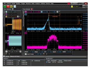
Mask tests, histograms and a wide variety of functions such as the gated FFTs in the above image provide deep signal analysis.
