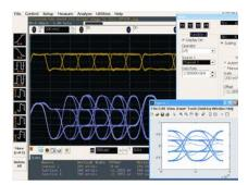
Signal equalization using user-defined function.
