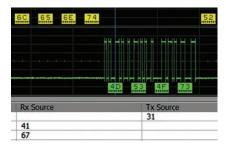
Trigger on and decode RS-232/UART transmission.
