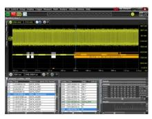
Trigger on and decode SATA serial packets.
