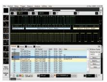
Trigger and view on-screen serial decode of  ${\rm I}^2 C$  packets.
