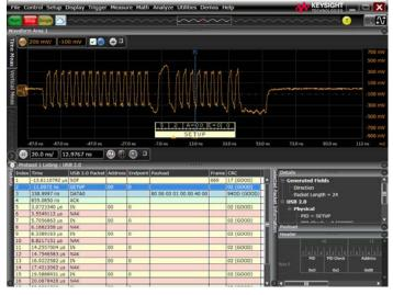
Quickly move between physical and protocol layer information using the time-correlated tracking marker. Display protocol content using waveform symbols and the industry's first multi-tab protocol viewer. The packets tab shows a high level view of the packet over time.
