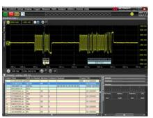
Trigger on and decode USB packets
