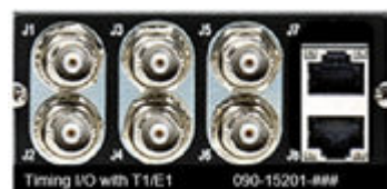
Figure 2-15. Timing I/O with Telecom I/O Connections (090-15201-011)
