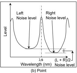
Figure 5.5.3-2 Detection Method for Noise Level
