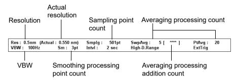
Figure 4.3-1 Measurement Condition Display Field
