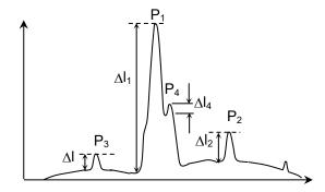
Figure 5.1.1-1 Example of Waveform where 2nd Peak Not Measured Correctly
