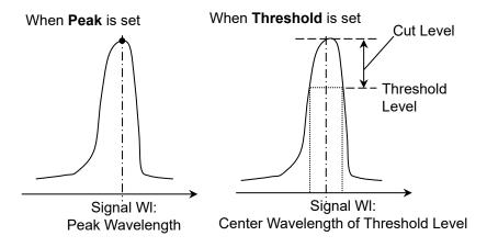
Figure 5.8.2-3 Signal Wavelength Measurement Method
