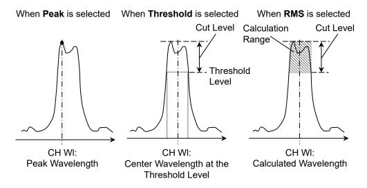
Figure 5.9.3-3 Measurement Method for Signal Wavelength
