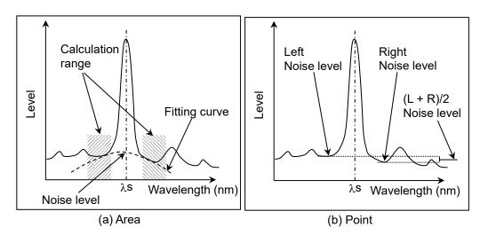
Figure 5.6.2-2 Detection Method for Noise Level
