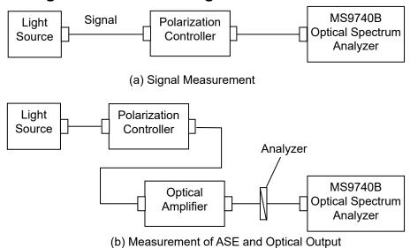
Figure 5.7.4-1 Measurement System for Polarization Nulling Method
