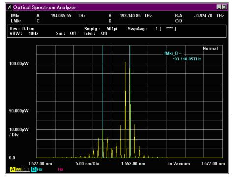
Figure 3.7.1-1 Waveform Marker Display
