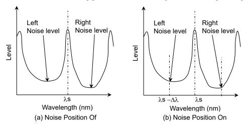
Figure 5.5.3-3 Measurement of Noise at Noise Position
