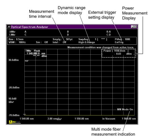
Figure 4.7-1 Measurement Settings Field and Power Measurement Display
