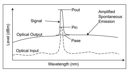
Figure 5.7.1-1 Level Measured with Optical Amplifier Measurement Function
