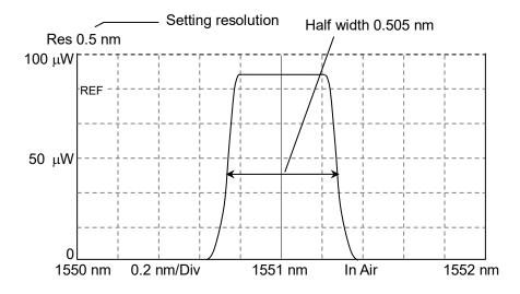
Figure 1.3-6 Measurement Example of Resolution 0.5 nm
