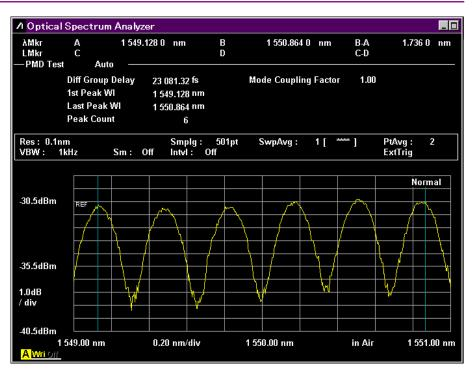
Figure 5.4-2 PMD-Test Example
