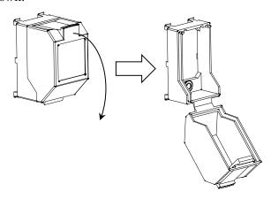
Figure 2.2.1-2 How to Opening the Optical Connector Cover
