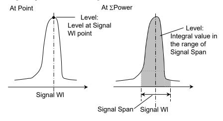
Figure 5.5.2-4 Measurement Method for Signal Level
