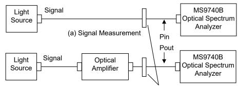
(b) Measurement of Optical Output Optical Bandpass Filter
