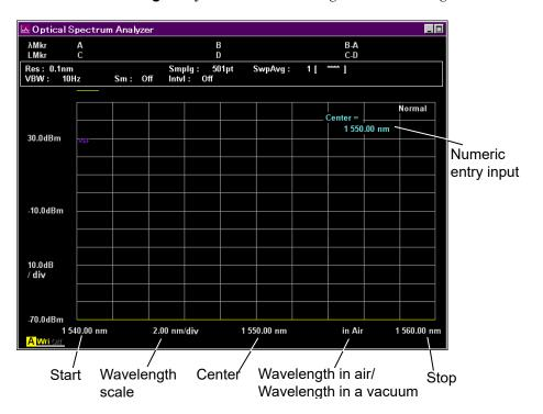
Figure 4.1-1 Names of Wavelength Display
