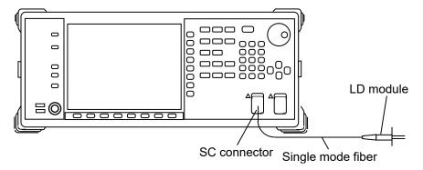
Figure 3.2-2 Connection Example of Laser Diode Module
