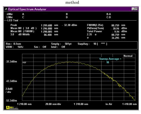
Figure 5.3-1 LED-Test Example
