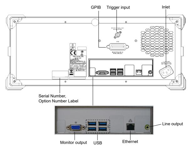
Figure 2.2.2-2 Rear Panel (MS9740B-108 and MS9740B-208)
