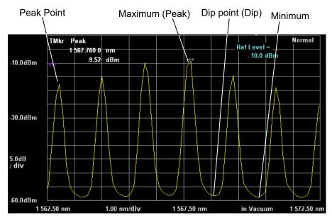
Figure 4.4-1 Waveform Peaks and Dips
