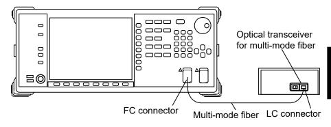
Figure 3.2-1 Connection Example of Optical Transceiver
