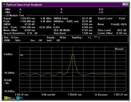
Figure 5.6-1 LD Module-Test Example
