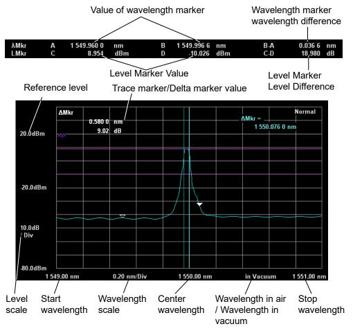
Figure 2.12-3 Marker, Level Scale, Wavelength Displays
