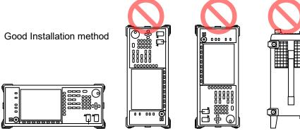
Figure 2.1.2-1 Installation Orientation
