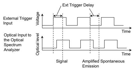
Figure 5.7.5-2 Definition of Ext Trigger Delay
