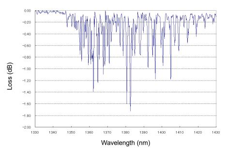
Figure 2.7-2 Water Vapor Absorption Spectrum
