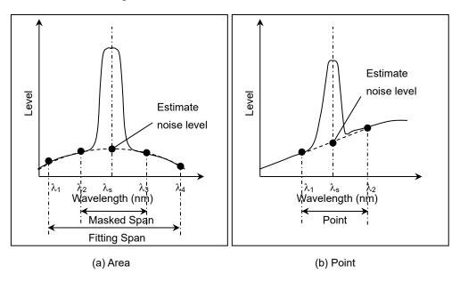
Figure 5.8.3-2 Detection Method for Estimated Noise Level
