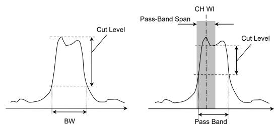
Figure 5.9.3-4 Measurement Method for Bandwidth
