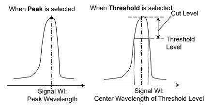
Figure 5.5.2-3 Measurement Method for Signal Wavelength
