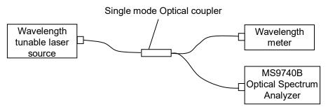
Figure 7.2.1-1 Wavelength Accuracy Test Setup
