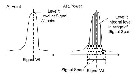
Figure 5.6.1-4 Measurement Method for Level
