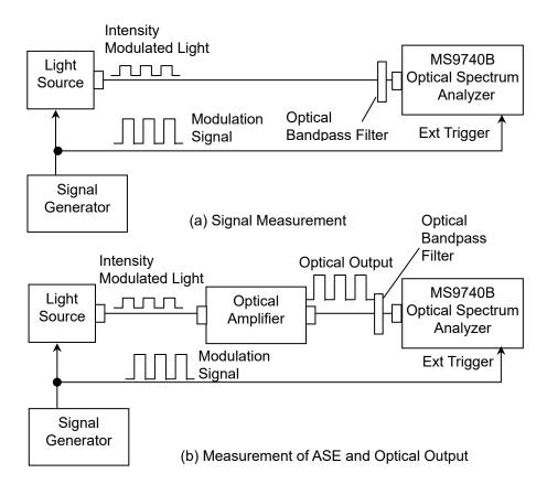
Figure 5.7.5-1 Pulse Method Measurement System
