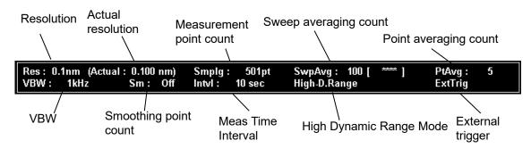
Figure 2.12-4 Measurement Condition Setting Display Field
