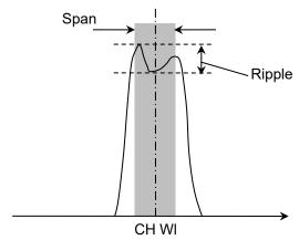
Figure 5.9.3-5 Measurement Method for Ripple
