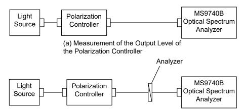
(b) Measurement of Analyzer Output Level
