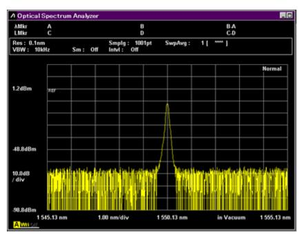
Figure 1.3-2 Example of Measurement at VBW 10kHz
