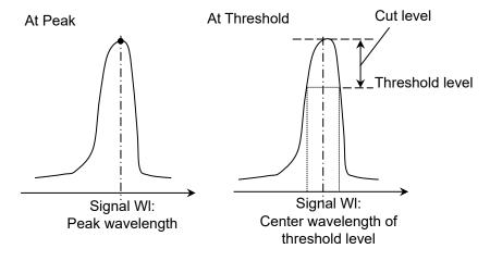
Figure 5.6.1-3 Measurement Method for Wavelength
