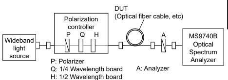
Figure 5.4.2-1 PMD Measurement System
