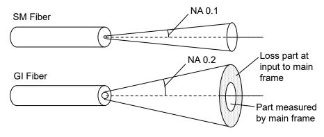
Figure 2.7-1 Difference in light radiated from optical fibers
