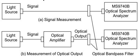
Figure 5.7.3-1 Optical Amplifier Measurement System
