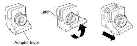
Figure 7.4-1 Cleaning the Ferrule End Surface 1
