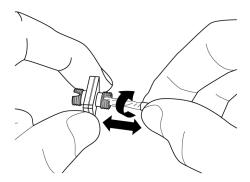
Figure 7.4-4 Cleaning the Ferrule End Surface 4
