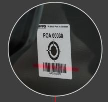
Built-in barcode scanner to link each asset to a Point of Attachment (POA) label for consistent measurements and trending within the OLPD Manager<sup>™</sup> Software
