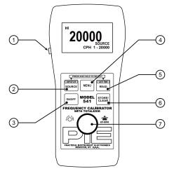
Turn the EZ-Dial knob  $\hat{O}$  to change the output frequency in increments of one least significant digit. Push down and turn for faster dialing with increments of 100 digits.
