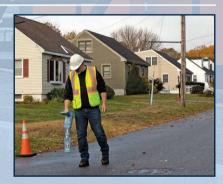
Cable sheath faults can be located to within 4" (10cm) using 8kHz Fault Find mode with a Radiodetection A-Frame.
