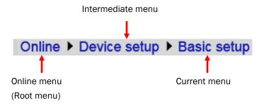
**Note:** The HART Menu Path bar also provides direct access to any of the menus along the menu path bar. Simply select the desired menu (touchscreen or arrow keys) from any displayed on the Path Bar and it will become the active menu.
