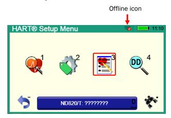
**Note:** The offline icon **②** covers part of the HART icon to indicate that you are no longer connected to a physical device.
