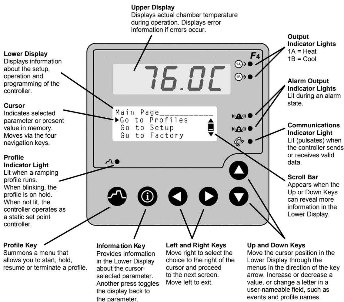
**Figure 4.1 – Temperature Controller Keys and Displays**
