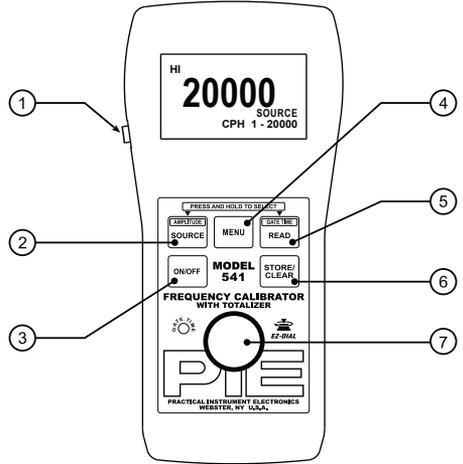
Turn the EZ-Dial knob ⑦ to change the output frequency in increments of one least significant digit. Push down and turn for faster dialing with increments of 100 digits.
