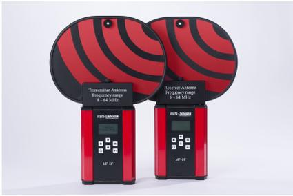
ETS-Lindgren's MF-9F Series of RF Leak Detector/Attenuation Meter Kits are designed to simplify the performance evaluation of shielding enclosures. These kits offer the ability to make measurements for military and commercial standards. The receiver module can store up to 63 attenuation levels per frequency to be downloaded to a PC. Windows compatible software is included for viewing, processing, and printing data.
