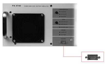
The "CONTROL" connector is an input port for the function generator; it can be directly connected to the appropriate connector at the function generator card of your **NSG series.**
