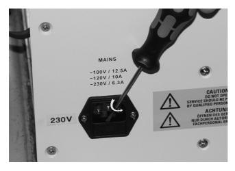
■ Pull out the drawer from the input connector assembly.
