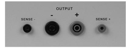
The output connectors of the PA 5740 series (back)
