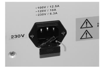
Remove the defect fuse.
