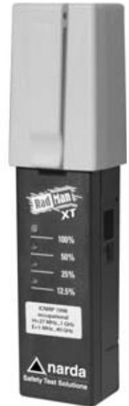
instrument with isotropic detection and four level indicator LEDs that provide an approximate indication of field strength. The RadMan can also be used as a simple area monitor. The fiber optic interface and available software can be used to continuously monitor the detected field strength levels from both the electric field and magnetic field sensors.
