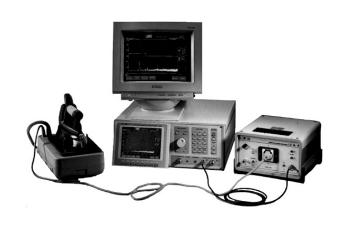
The "action" feature, for example, provides functionality of a complete automatic system without the need for an external PC. It can control LISNs, perform a sequence of measurements, find the worst case reading and print or save the desired results. This may be programmed, stored and then repeated, completely automatically, as many times as are needed with no need for an attending operator. The built-in hard disk and 3 ½ inch floppy drive give extra convenience to save, load or transport data.
