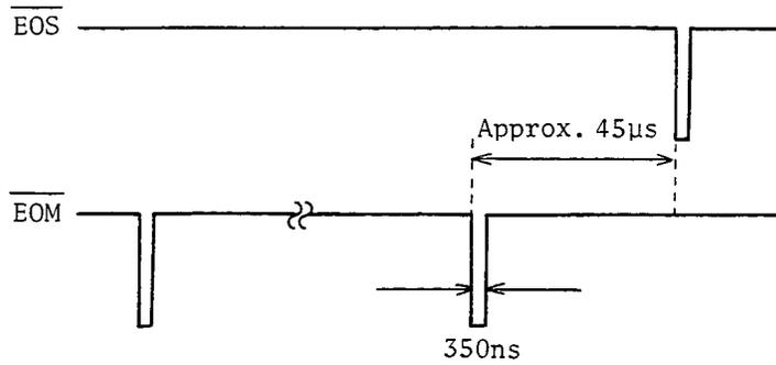
Figure 5-8.  $\overline{EOS}$  and  $\overline{EOM}$  Output Timing ( Typical )
