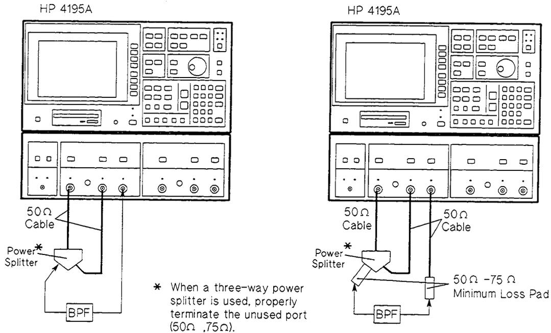
**50  $\Omega$  Device Measurements**
