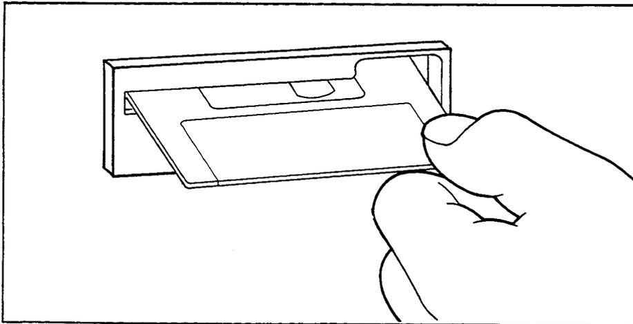
Figure 5-12. Proper Loading of the Flexible Disc
