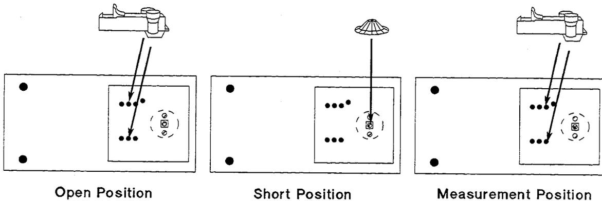
Figure 3-5. Attachment Connection
