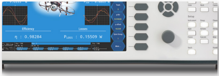
LMG triggers on data or commands from CAN bus and executes actions (e.g. starts a log)
