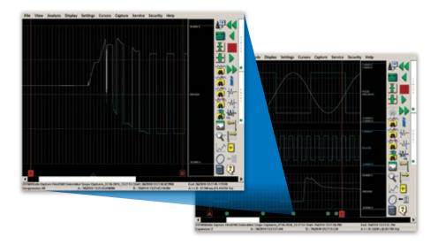
**Channel meters** allow users to view any channel as a digital readout, bar meter, moving needle, or analog gauge, making it easy to view current values at a glance. Users are able to visualize the relationships between inputs by plotting them in XYY plots. Channel meters and XYY plots can be sized and placed anywhere on the display for easy viewing.
