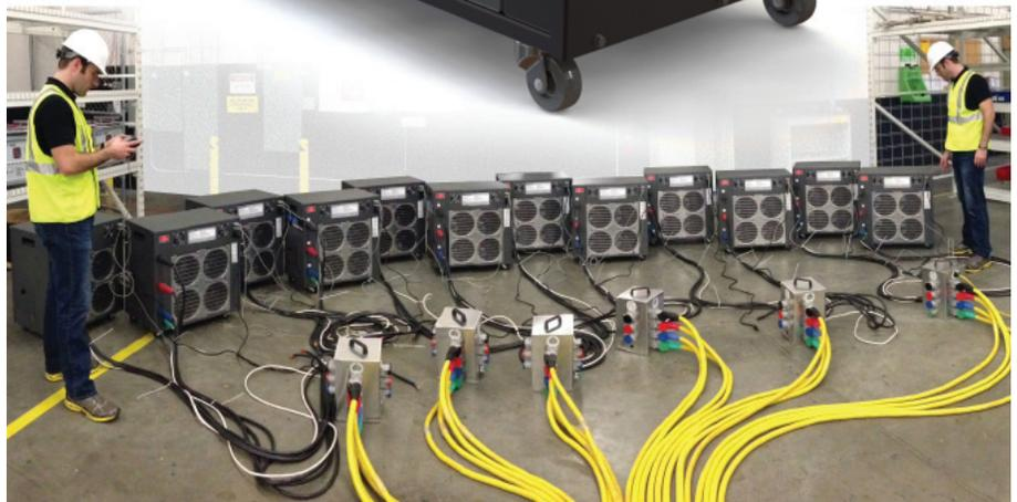
1800KW, 600V NorthStar Load Bank system formed by networking 12 NorthStar Units to a single Master Controller.
