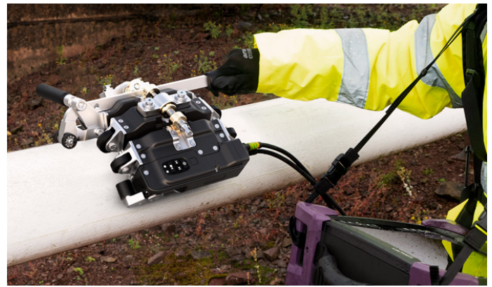
Figure 1: Pipescan HD deployment inspecting pipe for corrosion.
