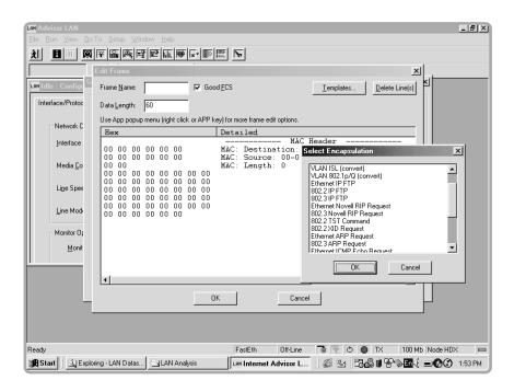
It provides intelligent packet and capture buffer file editing for full seven-layer customization of data to be transmitted. While you specify frame rate, burst count, or percent utilization, the software automatically calculates inter-packet gaps for various traffic loads, calculates the checksum and generates a CRC.
