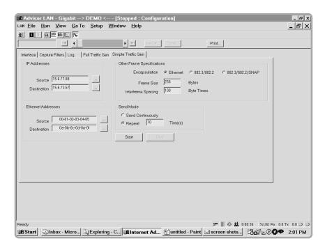
With the Gigabit Advisor traffic generator, each frame or pattern may be sent once (single shot) or in the automatic repeat mode with specified delay between each buffer (min. 1 usec). You can define the following parameters:
