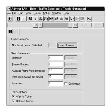
Frames from the capture buffer may be edited, then played back to duplicate hard-to-find problems. In addition, numerous message templates have been pre-defined for you. Detailed specifications for the traffic generator are provided below.
