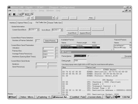
The traffic generator functions in the node mode only and while it is running, no other measurements are available.
