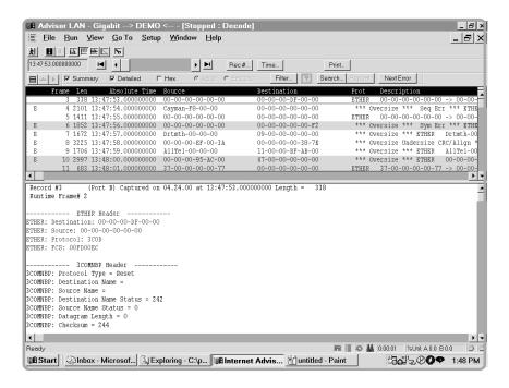
The Gigabit Advisor provides 7-layer decodes of all major protocols, including 802.1p, 802.1Q and 802.3x. For a complete list of decodes check our website www.agilent.com/comms/onenetworks
