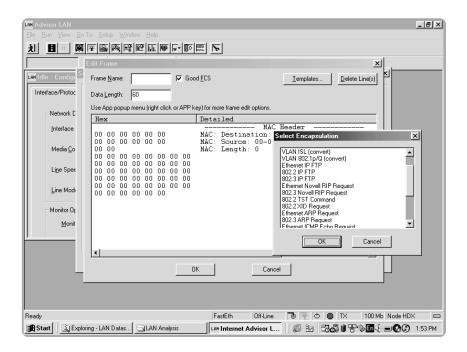
Frames from the capture buffer may be edited, then played back to duplicate hard-to-find problems. In addition, numerous message templates have been pre-defined for you. Detailed specifications for the traffic generator are provided below.
