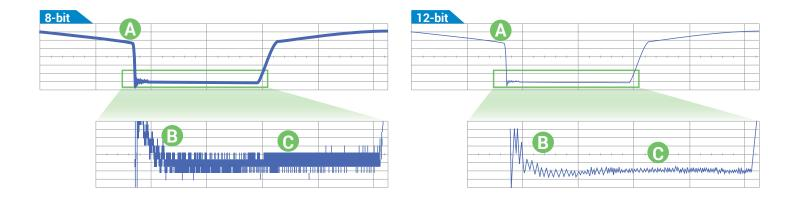
A Clean, Crisp Waveforms | Thin traces show the actual waveform with minimal noise interference
