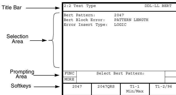
Figure 23 • DDS LL Setup Test Type View
