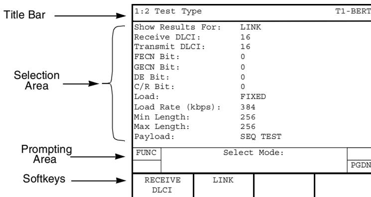
Figure 27 • Frame Relay Setup Test Type View
