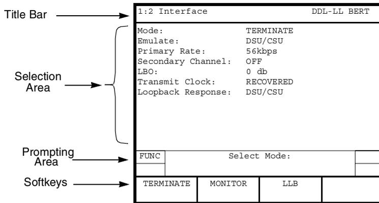
Figure 22 • DDS LL Setup Interface View
