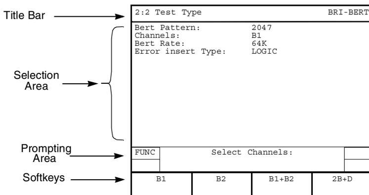
Figure 46 • ISDN BRI BERT Setup Test Type View
