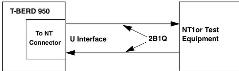
Figure 41 • ISDN BRI LT Terminate Mode
