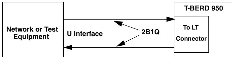
Figure 42 • ISDN BRI NT1 Terminate Mode
