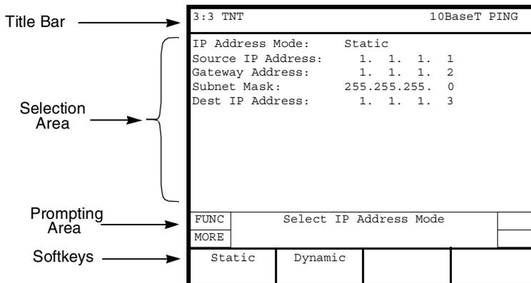
Figure 54 • 10BaseT TNT Setup View
