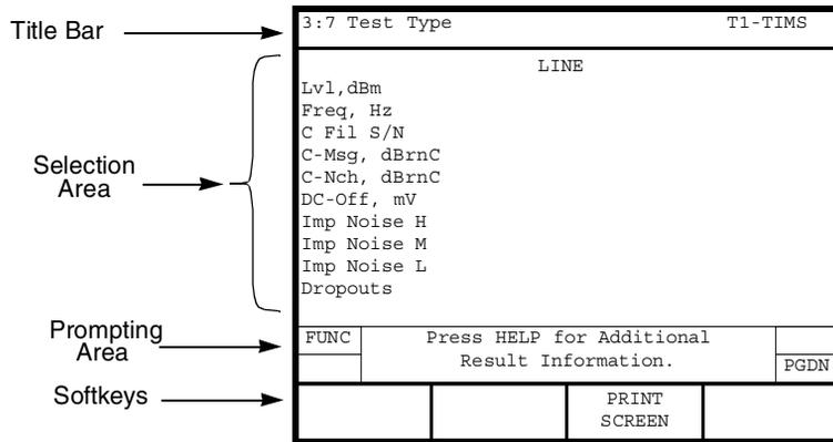
Figure 39 • PCM TIMS Test Type Results View
