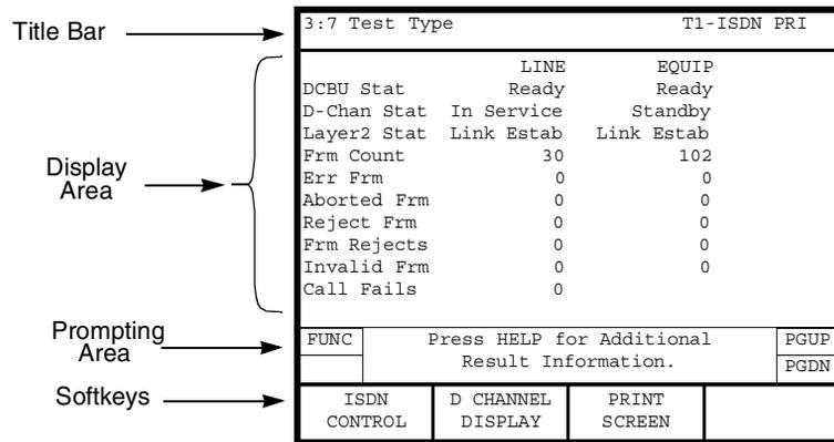
Figure 33 • ISDN PRI D-channel Backup Results
