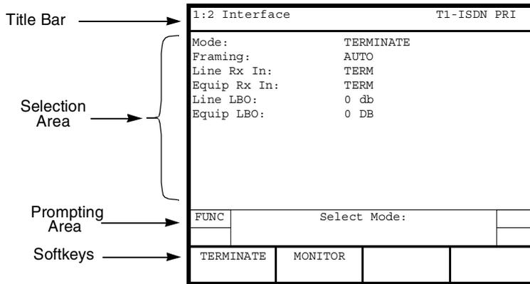
Figure 30 • ISDN PRI Setup Interface View
