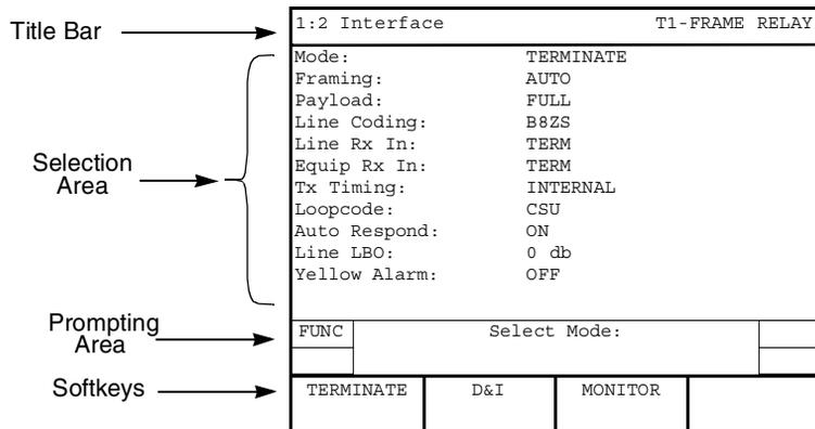
Figure 26 • Frame Relay Setup Interface View
