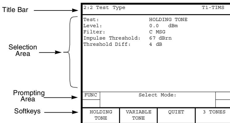
Figure 38 • PCM TIMS Setup Test Type View
