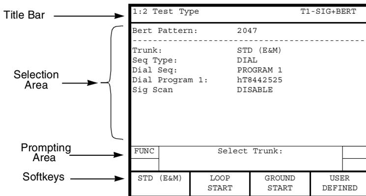
Figure 36 • Signaling Setup Test Type View
