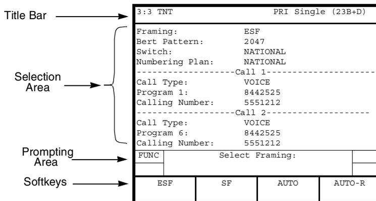
Figure 29 • ISDN PRI TNT Setup View
