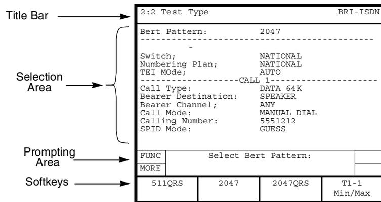
Figure 48 • ISDN BRI Test Type Setup View
