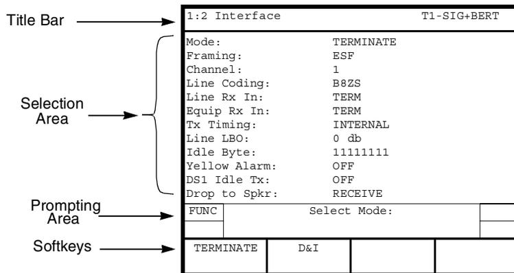
Figure 35 • Signaling Setup Interface View
