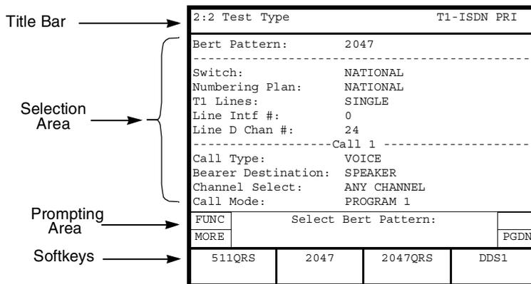
Figure 31 • ISDN PRI Setup Test Type View
