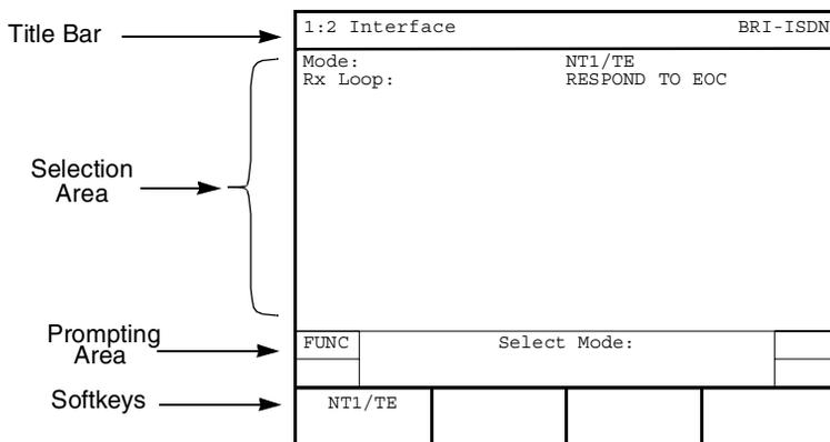
Figure 47 • ISDN BRI Setup Interface View
