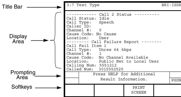
Figure 51 • ISDN BRI Call Status and Call Failure Report
