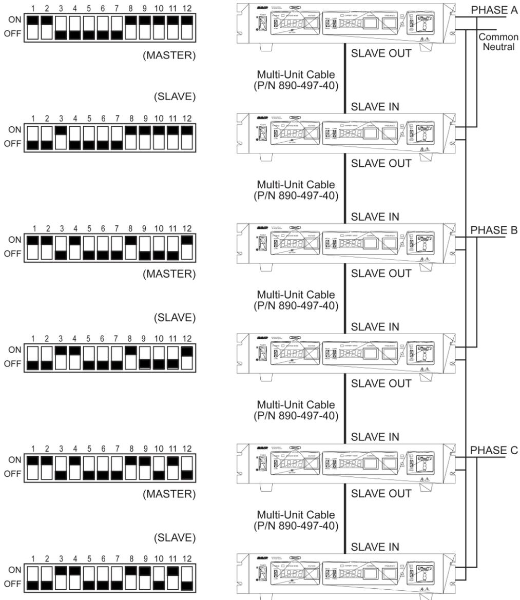
Figure 4-5. Dipswitch Settings for 3-Phase, 2-Paralleled Each, Configuration
