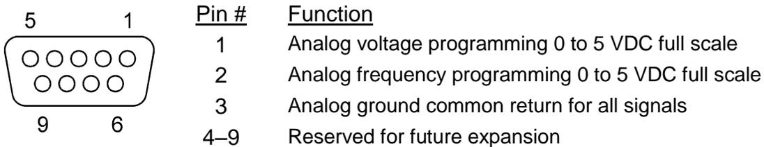
**Figure 5-2. External Control Connector**
