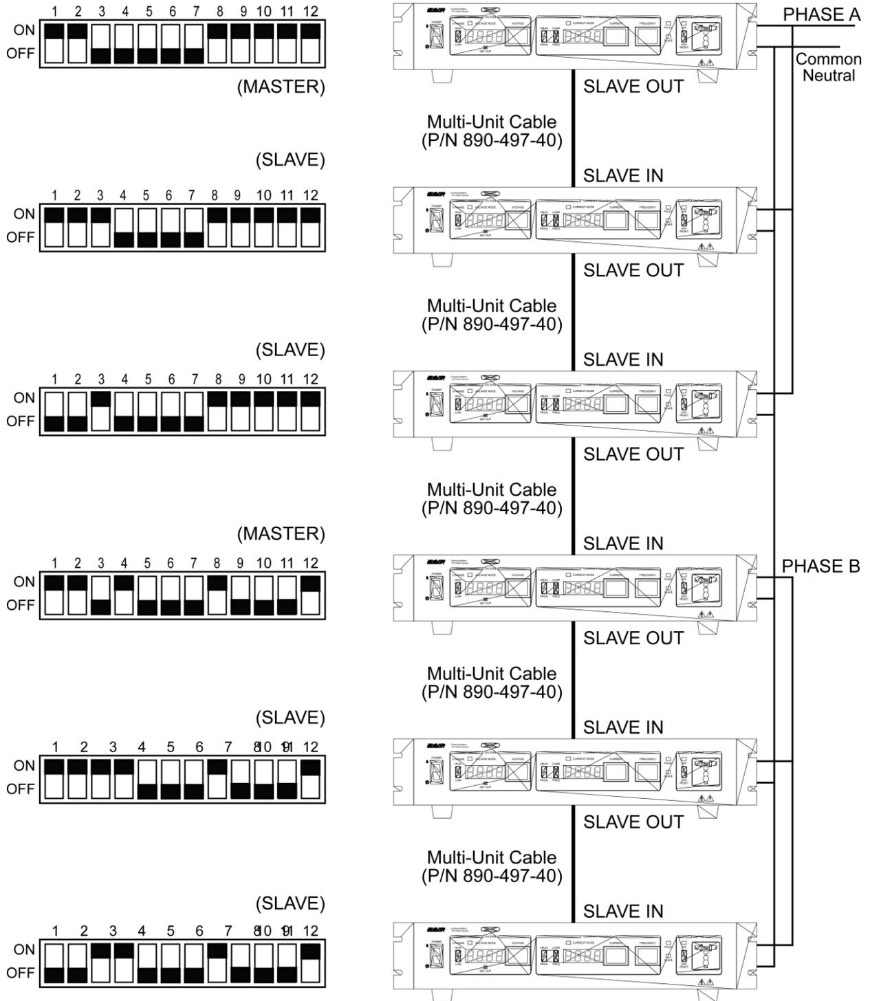
Figure 4-8. Dipswitch Settings for 2-Phase Configuration
