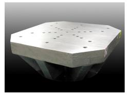
Carriage test specimen attachment plate
