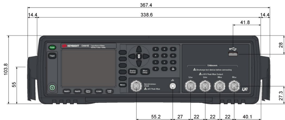
Figure 15. Dimensions (front view, with handle and bumper, in millimeters, nominal)
