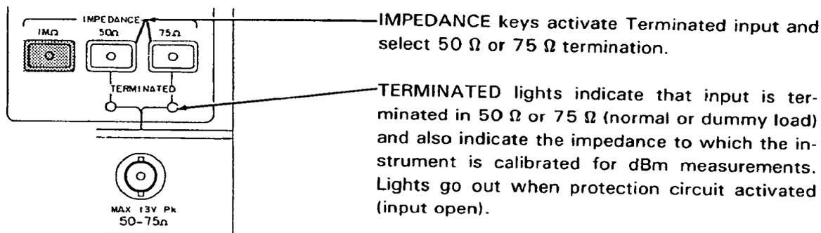
The Terminated input provides a 50-ohm or 75-ohm ( $\pm 1$  ohm) resistive termination. The dc-coupled terminating resistance is rated at one watt; specified return loss is  $> 26$  dB.\*
