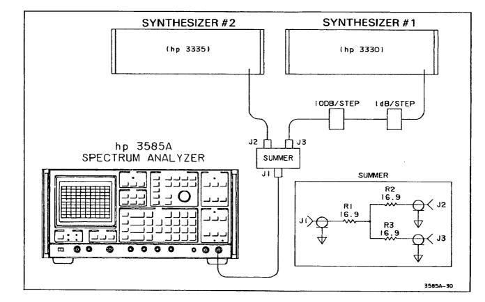
Figure 4-15. Intermodulation Distortion Test.
