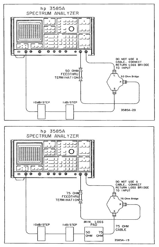
Figure 4-13. Terminated Input Return Loss Test (Automatic Tests).
