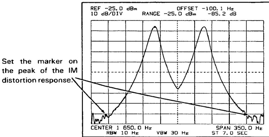
Figure 4-24. IM Distortion Response.
