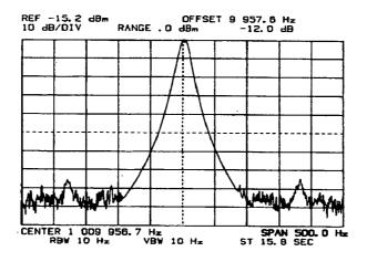
d. Narrow the Frequency Span about the Center Frequency to obtain the required resolution. Due to the change in Bandwidth and Sweep Time, the response may be skewed slightly off center, making it necessary to reposition the Marker. With the marker set to the peak of the response, move the response to the top of the screen by pressing [\_\_\_\_\_\_\_\_]. If you wish to measure succeeding harmonics in ''dB'' relative to the fundamental (rather than the carrier) press [\_\_\_\_\_\_\_].
