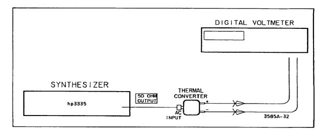
Figure 4-8. Measurement of Frequency Synthesizer For Calibration Data.
