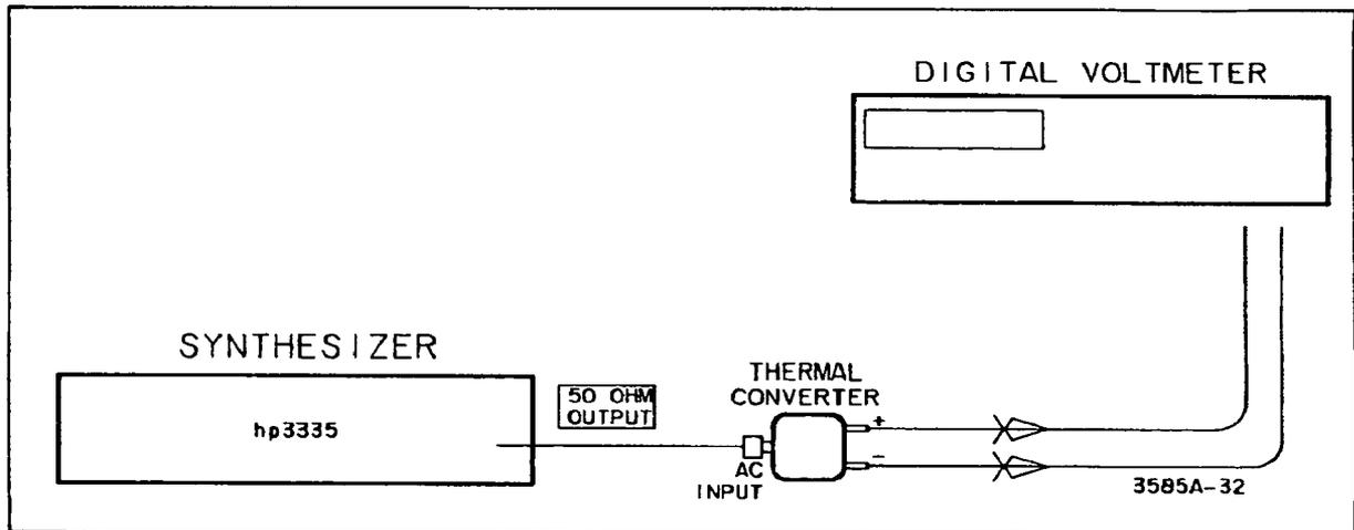
Figure 4-8. Measurement of Frequency Synthesizer For Calibration Data.
