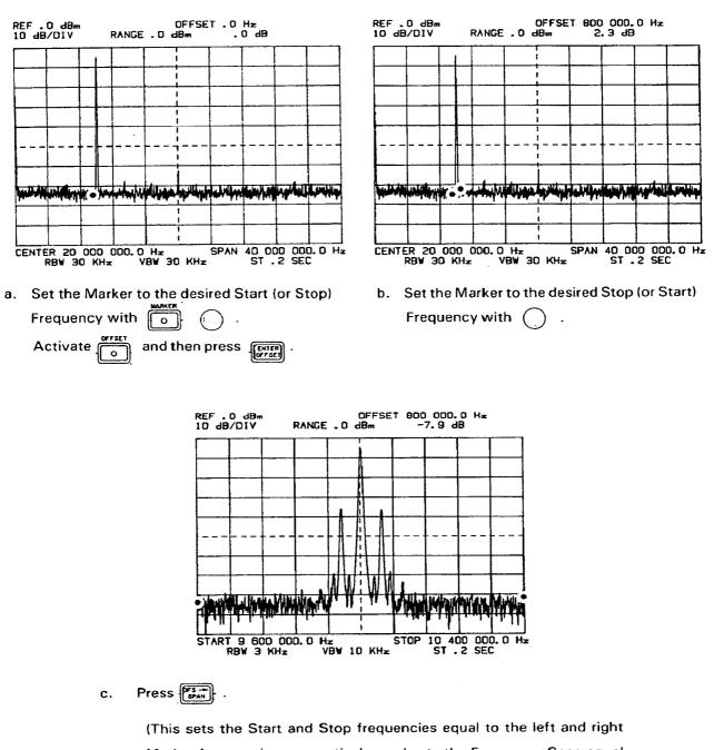
(This sets the Start and Stop frequencies equal to the left and right Marker frequencies, respectively; and sets the Frequency Span equal to the "OFFSET" frequency displayed in top-right corner of screen. Note that the Markers can be placed at either end of the Span. Pressing in automatically displays "START" and "STOP" in place of "CENTER" and "SPAN".)
