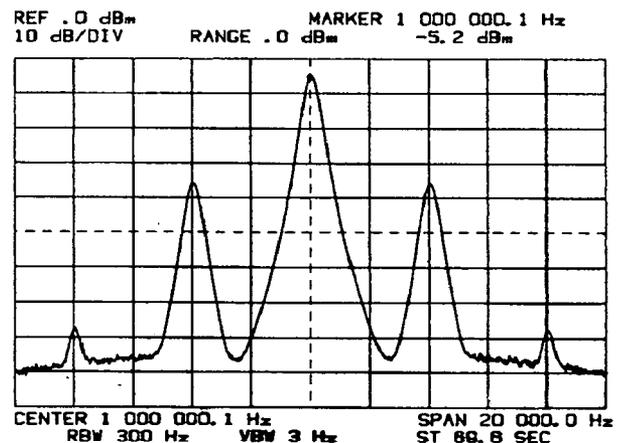
Narrowing VBW to 3 Hz (1% of RBW) reduces the noise variations, making it easy to see the low-level harmonics. (This also increased the Sweep Time and eliminated the frequency skew.)
