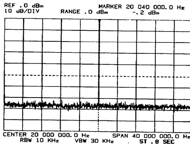
With optimum Sweep Time, 20.035 MHz response is skewed to the right and displayed at the 20.04 MHz point on the CRT trace.
