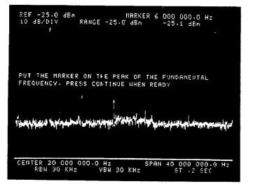
How the CRT looks after pressing RUN w/6MHz input.
