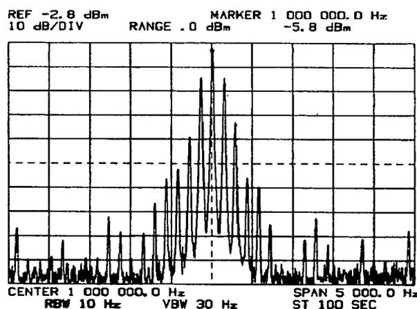
Signals resolved by narrowing RBW to 10 Hz (two steps); VBW tracks RBW; ST increases to 100 seconds to maintain absolute calibration.
