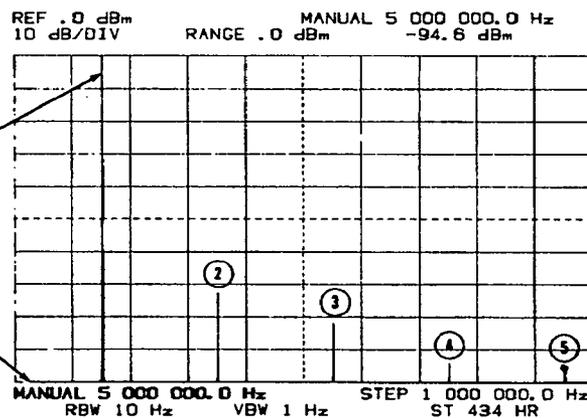
Low-Level harmonics of 1 MHz signal quickly measured with narrow bandwidth by stepping Manual frequency. Fifth harmonic is 94.6 dB below fundamental.
