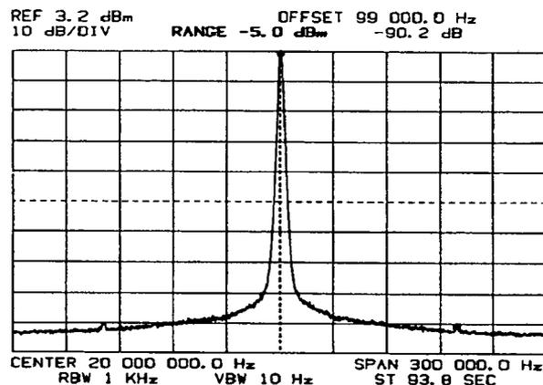
Decrementing the RANGE to -5 dBm (10 dB) reduces the internal noise level by 10 dB, providing a substantial improvement in the signal-to-noise ratio. The low-level spurious responses are still near the noise level of the external source; but the analyzer's internal noise is no longer contributing to the measurement.
