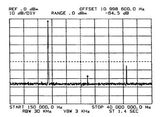
b. Set the Marker to the peak of the harmonic response with observe the "OFFSET" reading.
