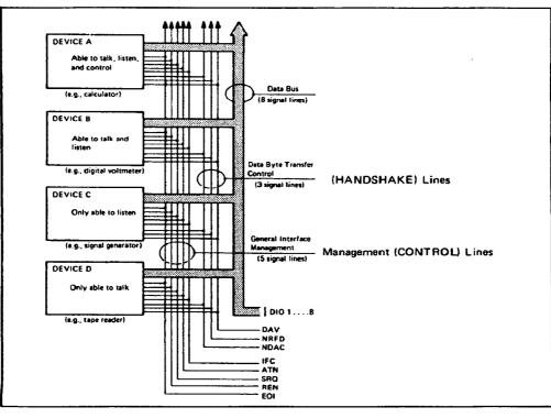
Figure 3-2-1. Interface Connections and Bus Structure.
