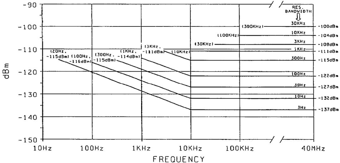
1 M $\Omega$  input: Below 500 kHz add 12 dB to above.
