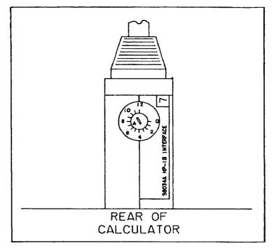
Figure 4-5. HP-IB Interface Cable Switch Setting.
