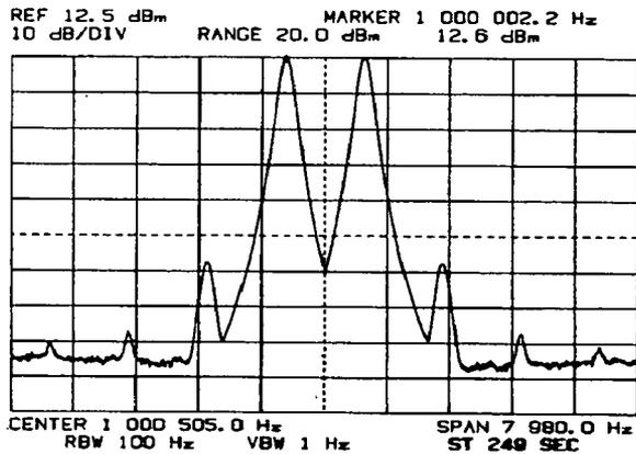
Driving Signals and Odd-Order IM Distortion Products.
