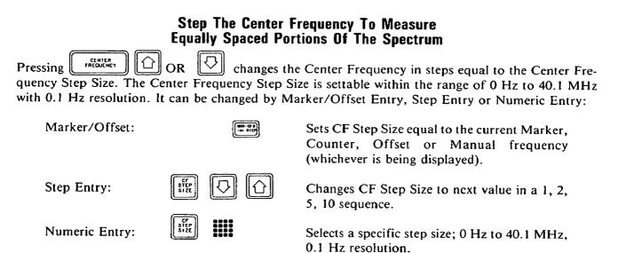
The ability to step the Center Frequency makes it possible to survey a wide frequency range in sequential pieces with high resolution. This is particularly useful for close-in observation of equally-spaced signals such as distortion products, modulation side frequencies, communication channels, etc. Here are some examples:
