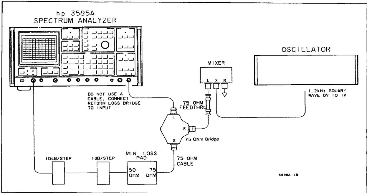
Figure 4-11. 75 ohm Return Loss Test (Automatic Tests).
