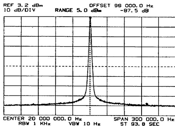
With RANGE set to +5 dBm, low-level spurious responses masked by the analyzer's internal noise *and* the noise of the external source are difficult to see and measure even with a narrow VBW.
