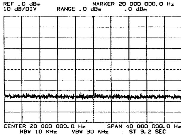
Sweep Time increased two steps to minimize frequency skew. Because of peak detection, 20.035 MHz response is now displayed at the 20.00 MHz point.
