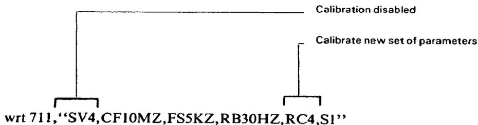
Example 3: Harmonic Distortion measurement using the Manual Mode.
