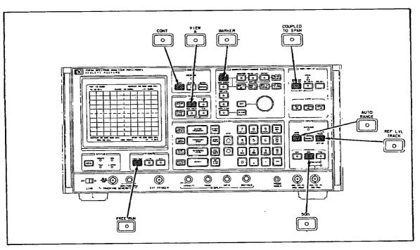
Figure 2-3. Front-Panel Functions Activated At Turn-On.
