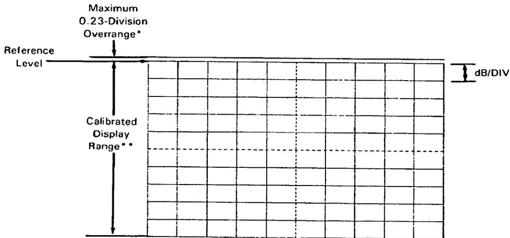
\*0.23 divisions = 2.3 dB, 1.15 dB, 0.46 dB or 0.23 dB; depending on the Vertical Scale (dB/DIV) setting. Amplitude accuracy is unspecified in this overrange region.
