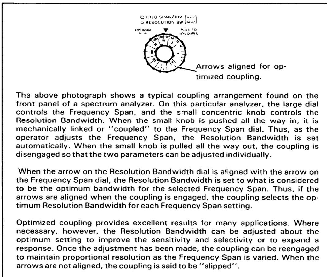
Figure 1. Mechanical Coupling.
