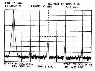
Prefacing the Start Frequency or Stop Frequency automatically displays the Start and Stop frequencies in place of Center and Span. The Start and Stop frequencies will continue to be displayed until Center Frequency, Frequency Span or CF Step Size is prefaced; Center Frequency is changed by Marker or Continuous Entry; a Manual frequency is entered or where or is pressed.
