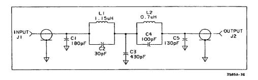
Figure 4-19. 9 MHz Low Pass Filter.
