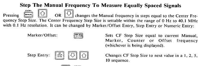
Selects specific step size; 0 Hz to 40.1 MHz, 0.1 Hz resolution.
