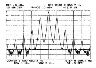
b. Set the Marker to the peak of the upper (or lower) side frequency. The "OFS CNTR" (Offset Counter) reading indicates the difference between the carrier frequency in the Offset Register and the counted side frequency on which the Marker is positioned. The amplitude readout indicates that the side frequency is 12 dB below the carrier.
