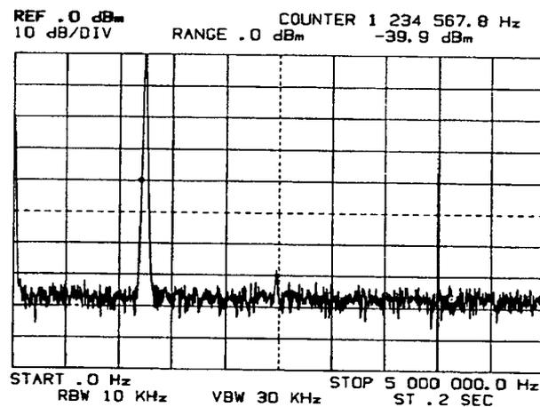
The "COUNTER" readout indicates the true signal frequency which applies to the peak of the response on which the Marker is positioned. (Note that the amplitude readout indicates the *Marker* amplitude rather than the peak amplitude.)
