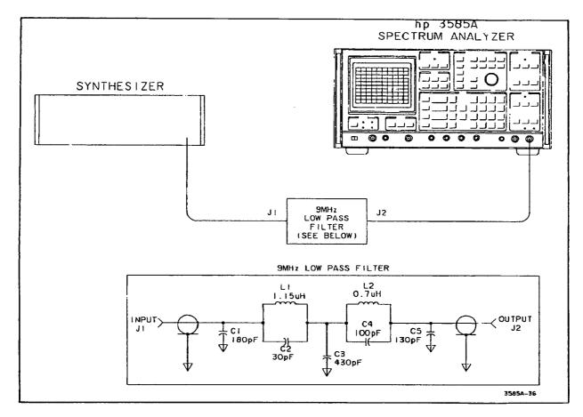
Figure 4-14. Harmonic Distortion Test
