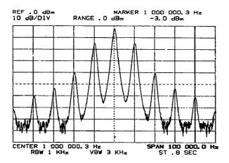
To individually measure the modulation side frequencies and harmonics with high resolution:
