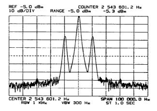
c. Narrow the Frequency Span about the Center Frequency to obtain the required resolution. If necessary, reposition the Marker to the peak of the response.
