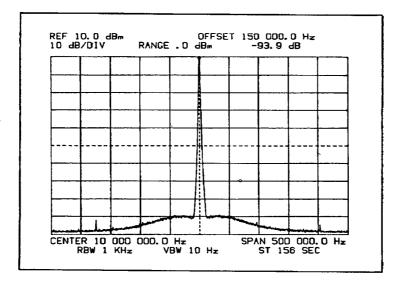
Figure D. Internal Phase Noise Pedestal
