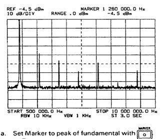
EXAMPLE: Measure harmonics in "dB" relative to the fundamental:
