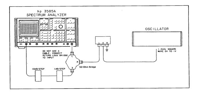
Figure 4-10. 50 ohm Return Loss Test (Automatic Tests).
