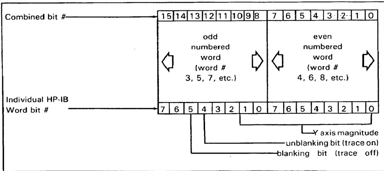
**Figure 3-2-3. CRT Trace Word In Binary Mode.**
