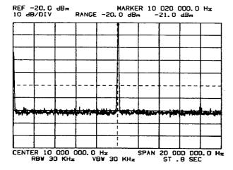
Peak of 10.035 MHz response displayed at 10.02 MHz point on CRT trace as indicated by "MARKER" frequency readout.
