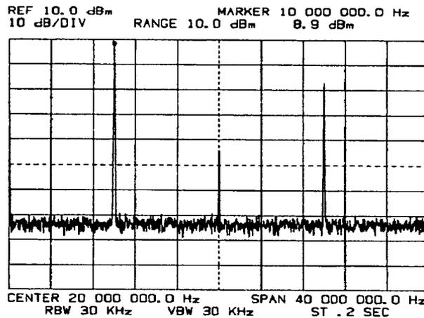
Measure absolute frequency and amplitude of on-screen responses with
