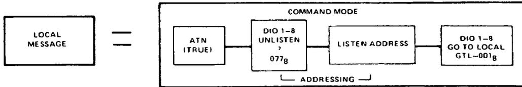
**LOCAL LOCKOUT.** The Local Lockout message prevents the operator from placing the instrument into local control from the front panel. The controller must be in the command mode to send the Local Lockout message.
