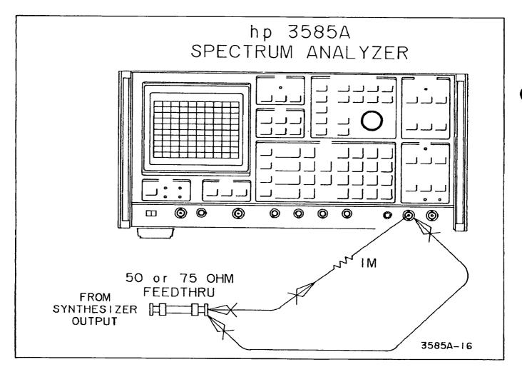
Figure 4-2. 1 M Ohm Input Impedance Test.
