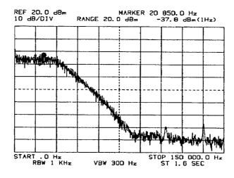
Noise level "dBm (1 Hz)" reading in top-right corner of screen indicates rms random noise spectral density at Marker, normalized to a 1 Hz noise power bandwidth.
