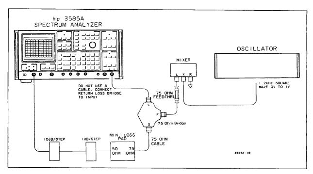
Figure 4-11. 75 ohm Return Loss Test (Automatic Tests).
