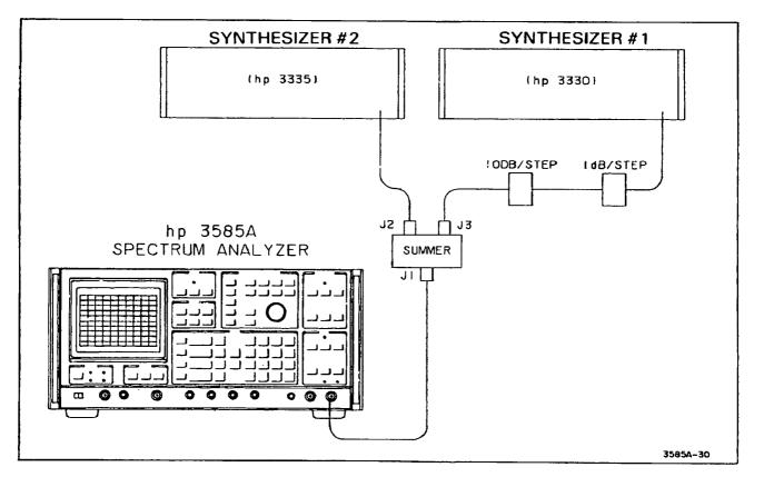
Figure 4-23. Intermodulation Distortion Test.
