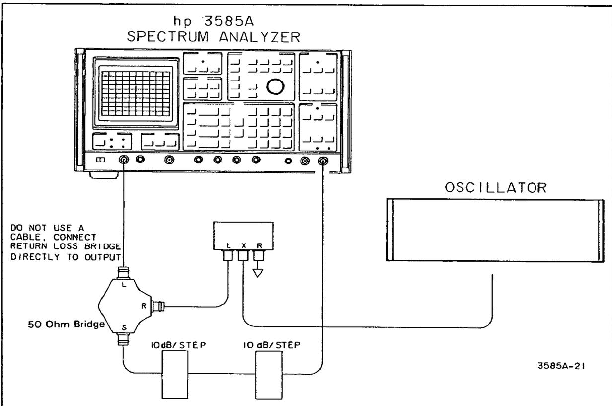
Figure 4-12. Tracking Generator Return Loss Test (Automatic Tests).
