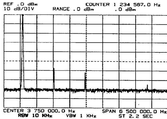
A single sweep with a 10 kHz RBW clearly shows the second and third harmonics of a 1.2 MHz signal. The fifth harmonic is visible but near the noise floor and the fourth harmonic is well below the noise. Narrowing the RBW to 10 Hz will reduce the noise by about 30 dB, enabling the fourth harmonic to be measured. All five harmonics can be quickly measured with a 10 Hz RBW by stepping the Manual frequency.
