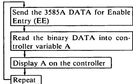
This program will display the decimal code for any key that is pressed. If a key is bad, the code displayed will not change when that key is pressed. If a key is stuck, only that key’s code will be displayed.
