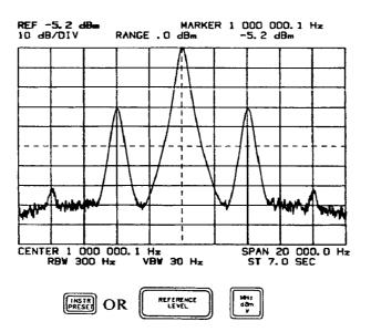
Displays REF, RANGE and Marker amplitude in "dBm" (50  $\Omega$  or 75  $\Omega$ ).
