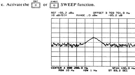
Fourth harmonic of 1.2 MHz signal measured in Manual mode (preceding example) moved to center of screen and displayed with 100 Hz Span. Reference Level lowered to -55.2 dBm to display the signal and noise on the CRT screen. (With the Reference Level at its original setting of 0 dBm, the noise is below the bottom graticule line and is not displayed.)
