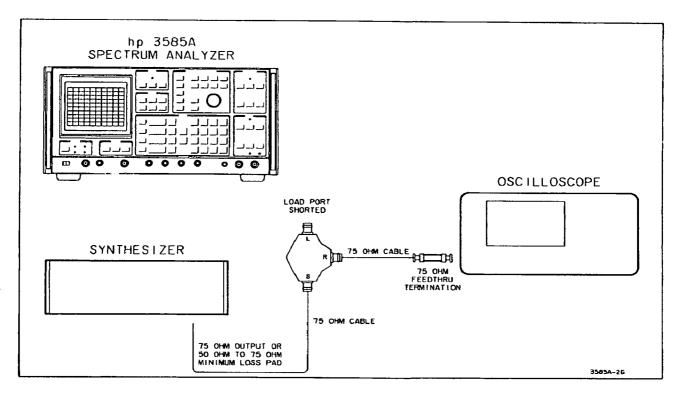
Figure 4-17. 75 $\Omega$  Return Loss Test (Operational Verification).
