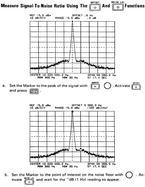
(The "dB (1 Hz) reading indicates the rms noise spectral density at the Marker in a 1 Hz bandwidth *relative* to the carrier amplitude.)
