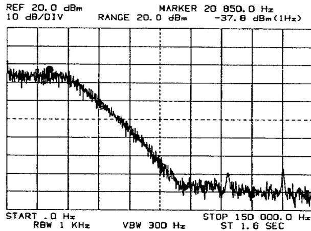
Noise level "dBm (1 Hz)" reading in top-right corner of screen indicates rms random noise spectral density at Marker, normalized to a 1 Hz noise power bandwidth.
