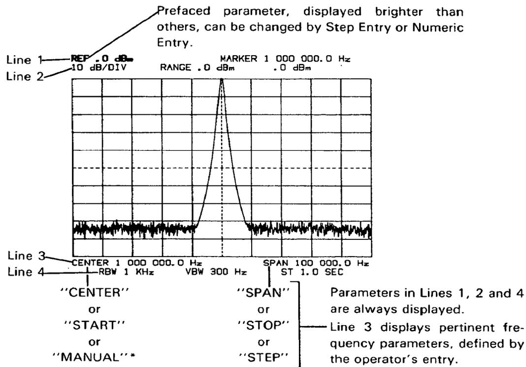
\* The Manual frequency is displayed here *only* when it is prefaced. The Manual frequency may also be displayed on the frequency readout in the upper right-hand corner of the screen.
