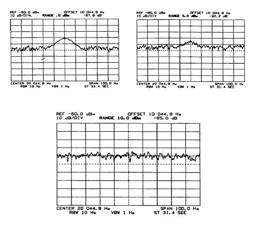
d. Incrementing the Range decreases the harmonic's amplitude, indicating that internal distortion is contributing to the measurement.
