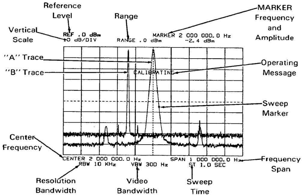
The CRT (Cathode Ray Tube) displays:
