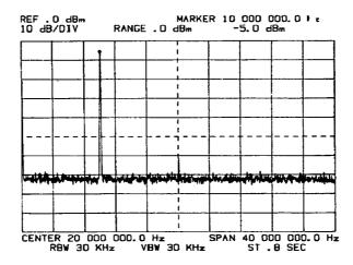
Marker at peak of 10.02 MHz response. During frequency sweep, peak displayed at 10.00 MHz point as indicated by "MARKER" readout.
