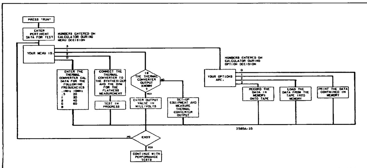
**Figure 4-6. Source Accuracy Program Flowchart.**
