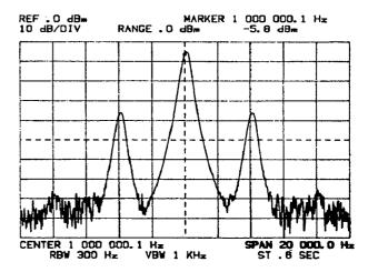
Frequency Span narrowed about Center frequency to obtain required resolution. RBW, VBW and ST parameters are set automatically.
