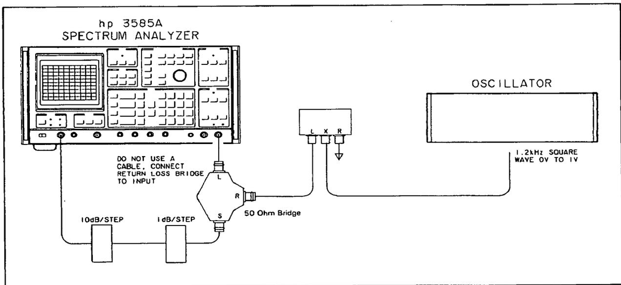
Figure 4-10. 50 ohm Return Loss Test (Automatic Tests).
