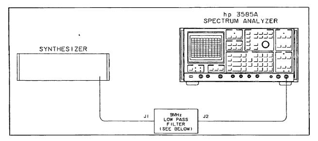
Figure 4-21. Harmonic Distortion Test.
