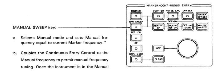
\*If the instrument is already in the Manual mode and the Marker is at the Manual measurement point on the CRT trace, pressing or activating will not change the Manual frequency.
