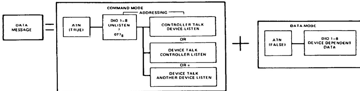
**TRIGGER.** The Trigger message causes all addressed instruments with this capability to execute some predefined function simultaneously.
