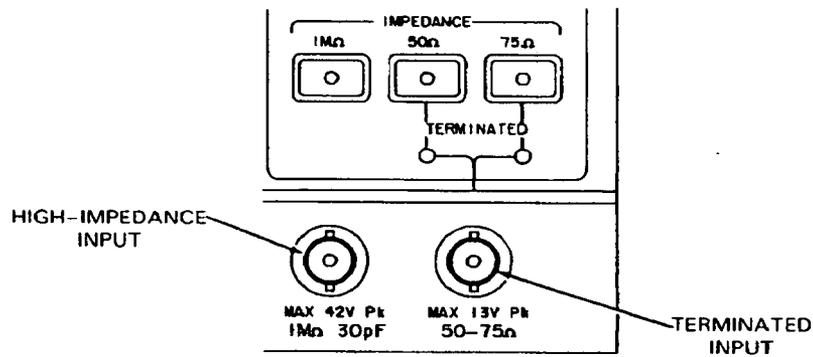
The inputs are mutually exclusive and, therefore, cannot be used simultaneously.
