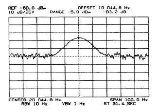
c. Second-harmonic response moved to center of screen and displayed with 100 Hz Span and 10 Hz RBW. Reference Level lowered to - 60 dBm to display signal and noise in upper portion of CRT screen.
