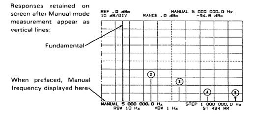
Low-Level harmonics of 1 MHz signal quickly measured with narrow bandwidth by stepping Manual frequency. Fifth harmonic is 94.6 dB below fundamental.
