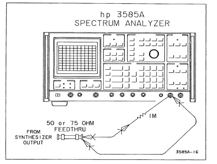
Figure 4-18. 1 M ohm Input Impedance Test.
