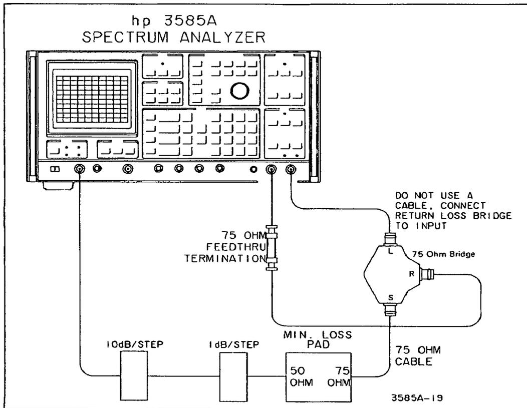
Figure 4-13. Terminated Input Return Loss Test (Automatic Tests).
