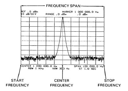
There are two basic methods for setting the frequency display range:
