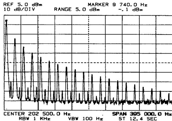
A single sweep over a 395 kHz Span displays the harmonic components of a 10 kHz triangle waveform. With the Resolution Bandwidth set to 1 kHz, many of the low-level even harmonics are too near the noise floor to be measured accurately. In the Manual mode, the harmonics can be individually measured using a narrow bandwidth.
