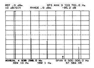
b. Clear the trace by pressing  $\begin{bmatrix} CLEAR \\ A \end{bmatrix}$ .
