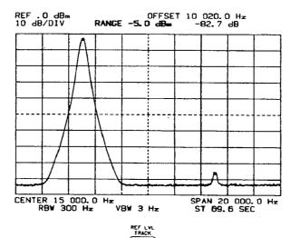
b. Downranging one step (with old decreases the internal noise level and increases the internal second-harmonic distortion making it easy to pinpoint the second-harmonic response.
