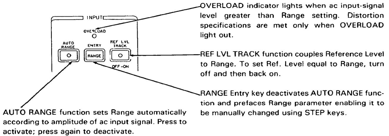
The Range setting determines the maximum ac signal level that can be applied to the Input (i.e., the input currently activated) without overdriving the input circuitry.
