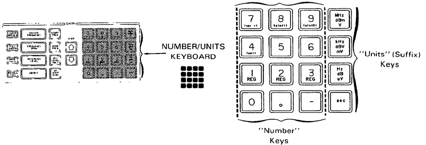
Numeric entries permit the operator to set the parameters to the exact values that are needed to make a specific measurement. While all of the major operating parameters (except Range) can be entered numerically, Numeric entries are used primarily to set the frequency parameters such as Center Frequency and Frequency Span or Start and Stop.
