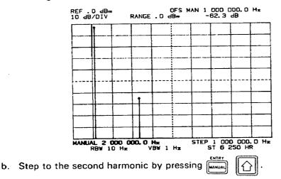
(A stationary Marker remains at the peak of the fundamental response; i.e., the point where pressed. The "OFS MAN" (Offset Manual) readout indicates the difference between the current Manual frequency and the frequency in the Offset Register. The amplitude readout indicates the harmonic's amplitude in "dB" relative to the amplitude in the Offset Register which, in this case, is the amplitude at the peak of the fundamental response.)
