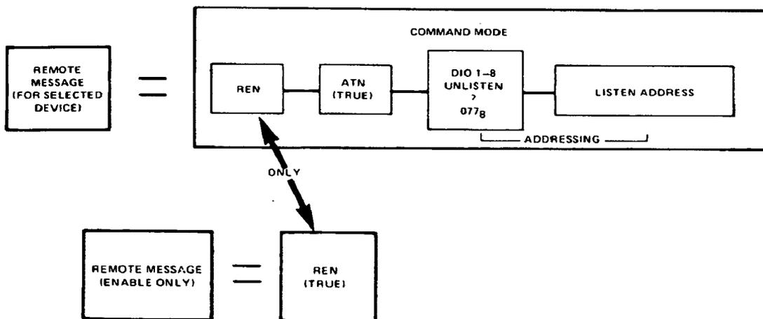
**LOCAL.** The Local message will remove addressed devices from the Remote operating mode to local (front panel) control. The controller must place the HP-IB into the command mode and address to listen all devices that are to be returned to local. The Local message does not remove the HP-IB from the Remote mode, only the listening devices.
