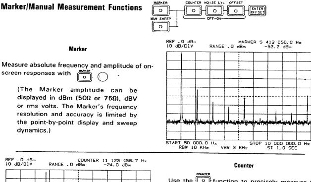
Use the of function to precisely measure the frequency of the signal that is producing the response on which the Marker is positioned.
