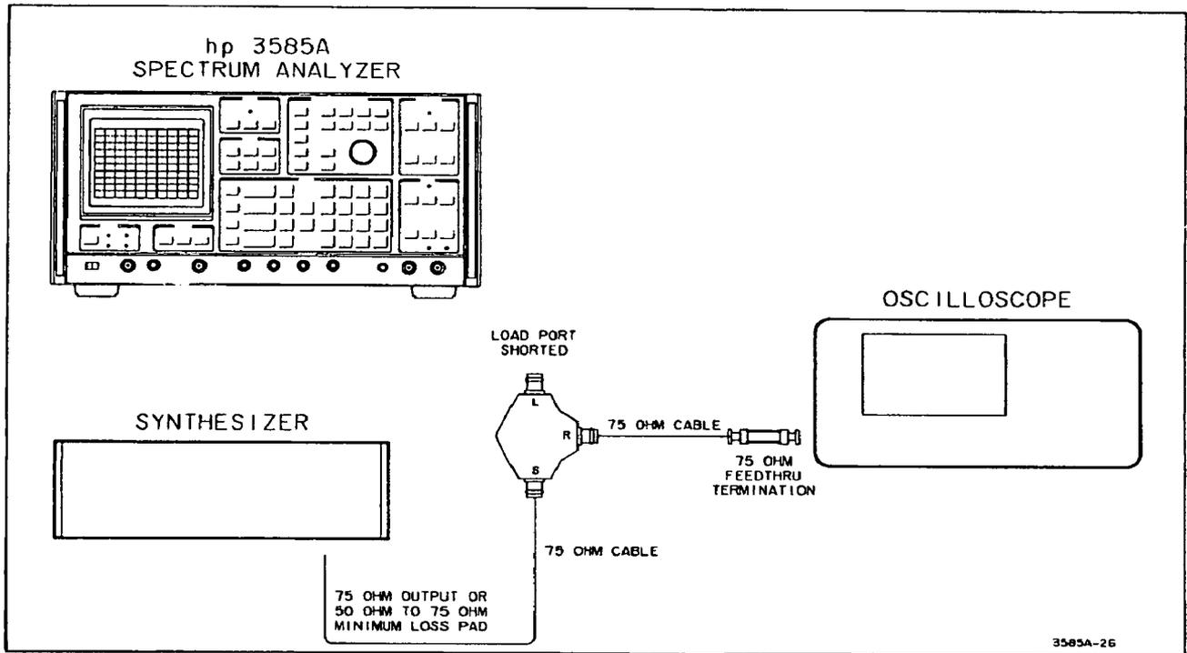
**Figure 4-17. 75Ω Return Loss Test (Operational Verification).**
