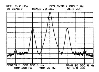
b. Set the Marker to the peak of the upper (or lower) sideband with O. Allow time for the "OFS CNTR" reading to appear. As indicated by the "OFS CNTR" reading, the true difference frequency is 4,003.5 Hz as opposed to the 4,000.0 Hz reading obtained in the preceding example.
