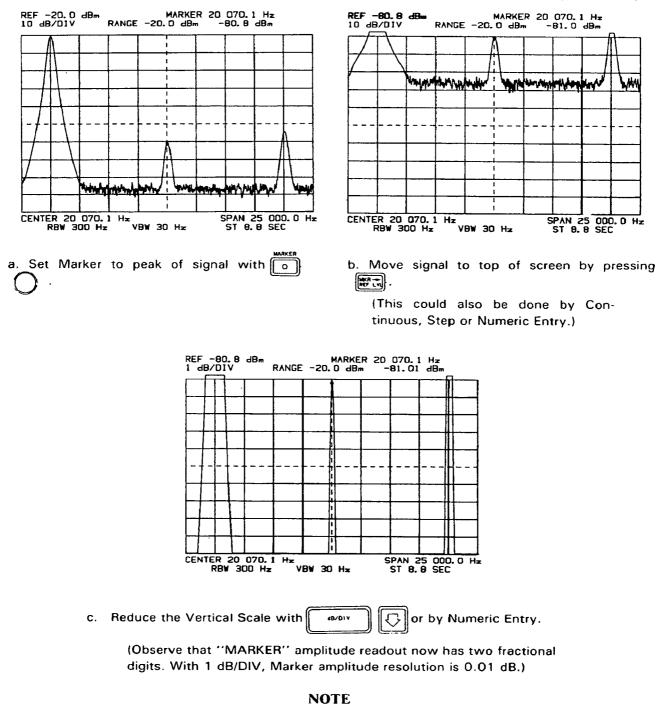
Here is a technique for moving a signal of interest to the top of the screen and expanding it vertically:
