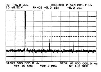
a. Set the Marker to the peak of the fundamental with . Move the fundamental to the top of the screen by pressing . Activate . Activate . to precisely measure the fundamental frequency.
