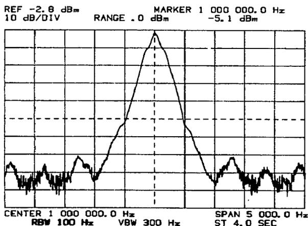
Closely spaced signals in 5 kHz Span unresolved with 100 Hz RBW (automatically selected).
