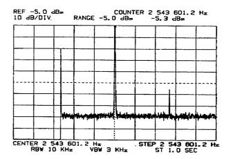
b. Move the fundamental to the center of the screen by pressing for by numerically setting the Center Frequency equal to "COUNTER"). Set the Center Frequency Step Size equal to the fundamental frequency (i.e., "COUNTER" frequency) by pressing for by Numeric Entry.
