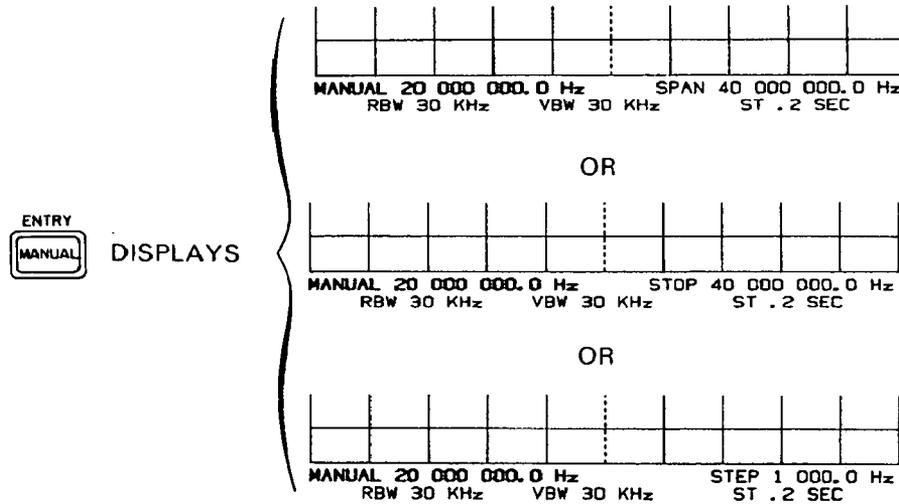
When the "MANUAL" entry is terminated, the display reverts to "CENTER" and "SPAN":
