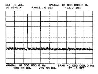
Pressing with second sets Manual frequency equal to Marker frequency. "MANUAL" readout in top-right corner indicates Manual frequency and real-time signal amplitude at Manual frequency. (The true frequency of the signal is 10.02 MHz rather than 10.00 MHz. To measure its peak amplitude, the Manual frequency must be fine tuned to 10.02 MHz. This can be done with with second sets.)
