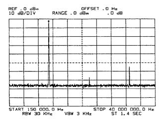
a. Set the Marker to the peak of the fundamental response with activate or activate or and then press (Entitient) -
