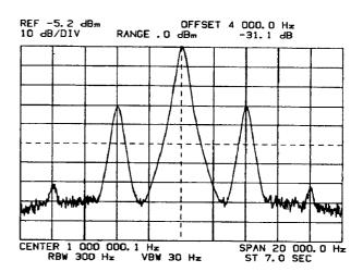
b. Set the Marker to the peak of the upper (or lower) sideband with O. (A stationary marker remains at the carrier frequency.) The "OFFSET" reading indicates the frequency and amplitude of the sideband relative to the carrier.\*
