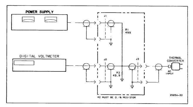
Figure 4.7. Thermal Converter Output Calibration.
