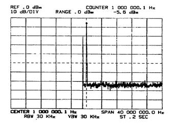
(This sets the Center Frequency equal to the ''COUNTER'' frequency.)
