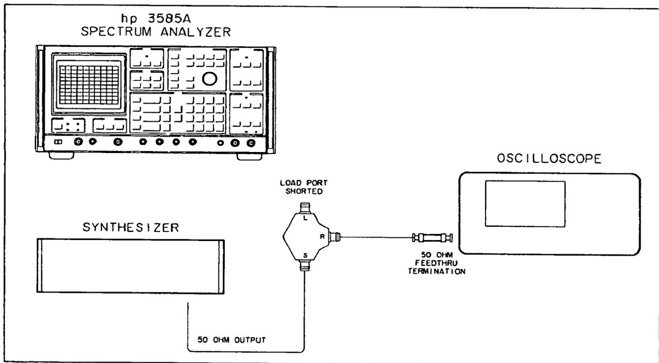
Figure 4-16. 50 $\Omega$  Return Loss Test (Operational Verification).
