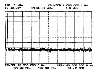
a. With and activated, set the Marker at least 20 dB above the noise floor on the skirt (or peak) of the response that is to be moved to the center of the screen. Allow time for the ''COUNTER'' reading to appear in the top-right corner of the screen.
