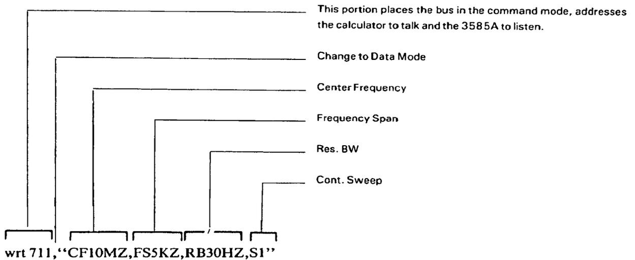
Example 2: This programming statement executes the same commands as the statement in Example 1; however, in this example the command string is written in accordance with the maximum programming speed guidelines of Paragraph 3.2.72. Try both Example 1 and 2 and note the difference in programming time.
