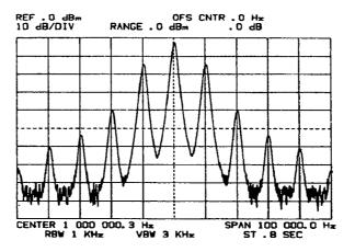
a. Set the Marker to the peak of the carrier with o. Activate of to precisely measure the carrier frequency. Store the carrier frequency and amplitude in the Offset Register by activating of and pressing of the carrier.
