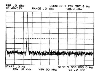
The "COUNTER" readout indicates the true signal frequency which applies to the peak of the response on which the Marker is positioned. (Note that the amplitude readout indicates the *Marker* amplitude rather than the peak amplitude.)
