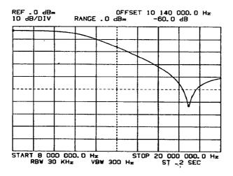
A frequency sweep from 8 MHz to 20 MHz displays the stopband response of a 9 MHz low-pass filter.
