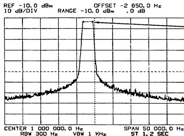
Trace plotted with MAX HOLD shows frequency drift of signal source during its 5-minute warmup.
