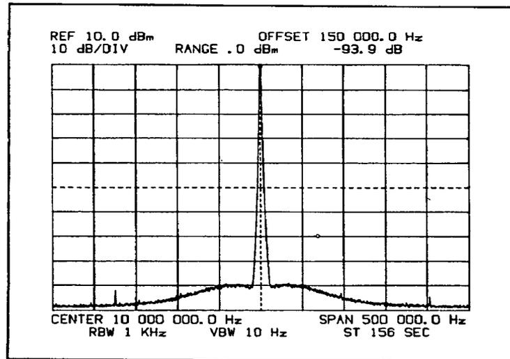
Figure D. Internal Phase-Noise Pedestal
