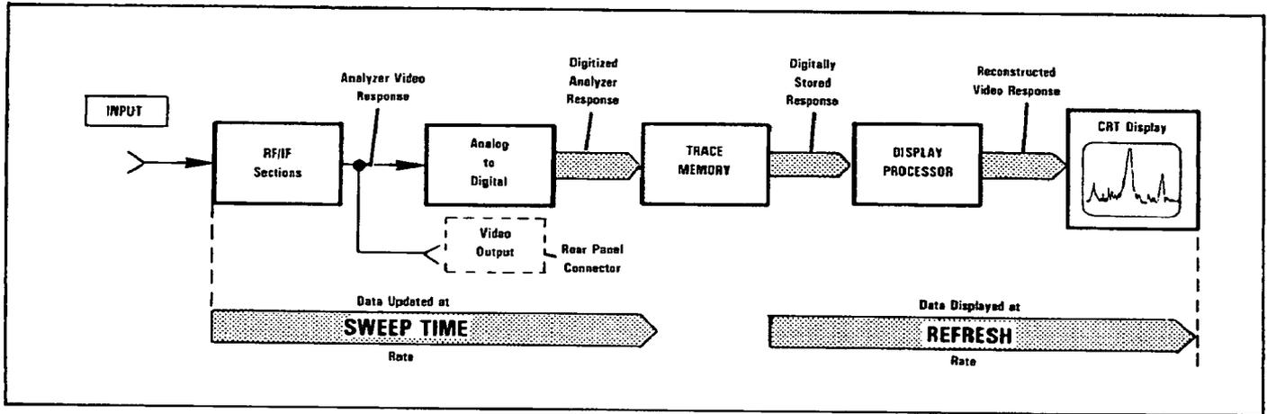
The above figure is a simplified block diagram showing the main signal path from the Input connector to the CRT display. The RF and IF sections of the analyzer comprise a swept superhetrodyne receiver whose output is a dc voltage that is logarithmically proportional to the input-signal amplitude. This dc voltage or "video response" is applied to the Analog-to-Digital (A/D) Converter where it is peak detected, sampled and transferred to the Trace Memory at a rate proportional to the Sweep Time.
