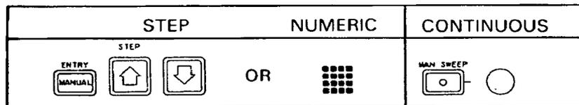
**Center Frequency Step Size (STEP).** The Center Frequency and Manual frequency can be incremented or decremented using the STEP keys. The Center-Frequency Step Size parameter sets the Center-Frequency *and* Manual-Frequency step size.
