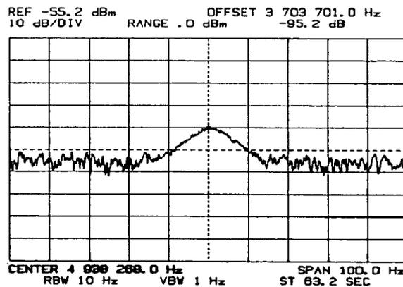
Fourth harmonic of 1.2 MHz signal measured in Manual mode (preceding example) moved to center of screen and displayed with 100 Hz Span. Reference Level lowered to -55.2 dBm to display the signal and noise on the CRT screen. (With the Reference Level at its original setting of 0 dBm, the noise is below the bottom graticule line and is not displayed.)
