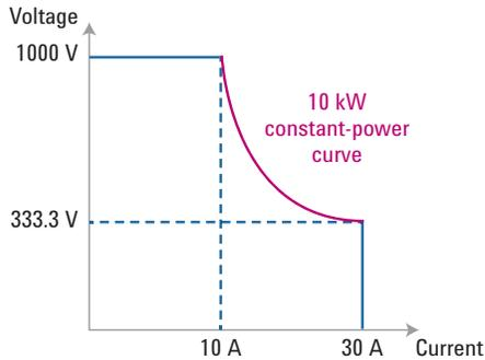
Figure 1. Autoranging output characteristic
