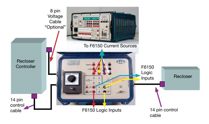
In this mode the simulated trip and close coils in the F5814 are bypassed and the F5814 simply passes the signal that it receives from the controller to the recloser trip and close coils. However, it still registers the trip and close status and passes this information to the F6150. The testing regimen conducted in the OPERATE mode are similar to the SIMULATE mode.
