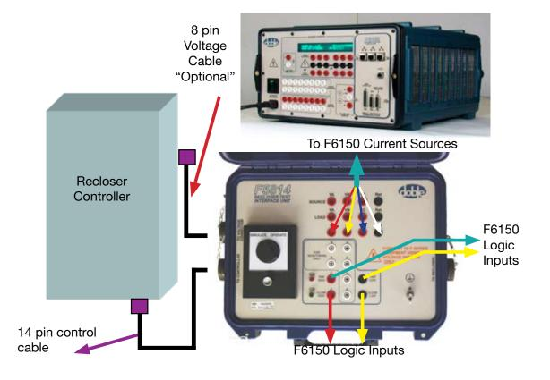
In this mode, the recloser is out of the circuit and hence the trip and close coils which are located in the recloser have to be simulated and this simulation is performed in the F5814. These simulated coils located in the F5814 react to the 24 Vdc that is provided by the recloser controller via the 14 pin control cable.
