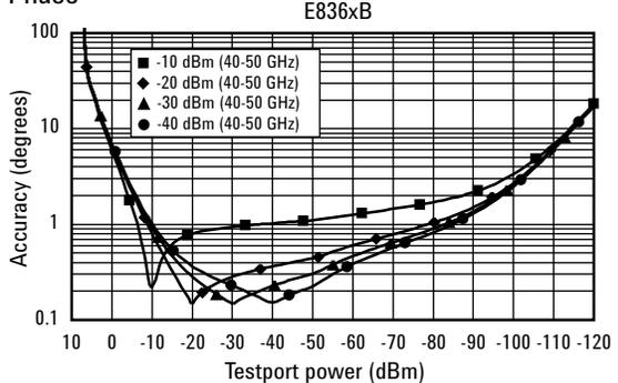
1. Dynamic accuracy is verified with the following measurements: compression over frequency, IF linearity at a single frequency of 1.195 GHz and a reference level of -20 dBm for an input power range of 0 to -120 dBm.
