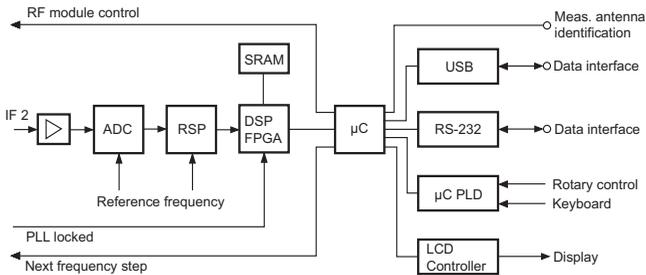
Fig. B-2 Block circuit diagram of main board
