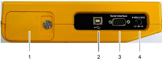
Fig. 6-4 Battery holder and external connectors
