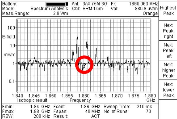
Fig. 8-20 Peak marker in the measurement menu
