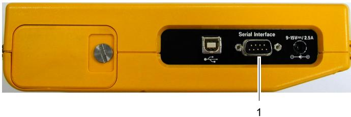
Fig. 16-2 Serial (1) and USB (2) interfaces
