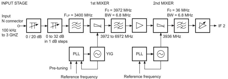
Fig. B-1 Block circuit diagram of RF module
