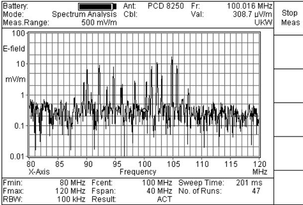
Fig. 11-7 “Spectrum Analysis” mode; separate sequential measurement
