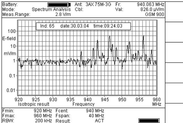
Fig. 13-9 Display of a stored data set using the MEMORY VIEWER
