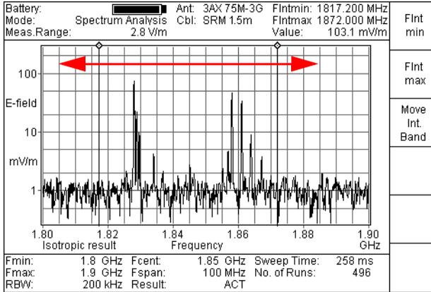
Fig. 8-30 Moving the frequency band
