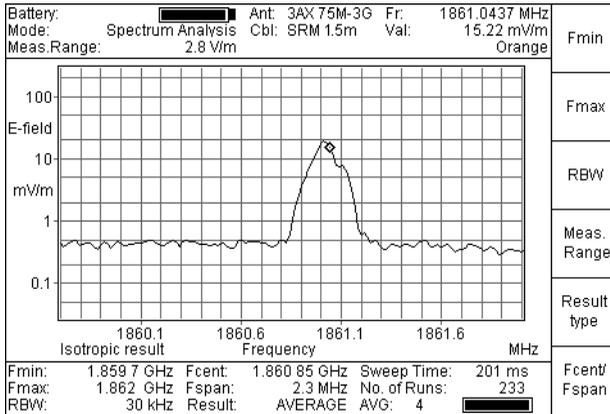
Fig. 8-19 Measurement menu after pressing the **Exec Zoom** softkey
