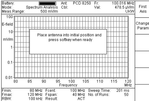
Fig. 11-6 "Spectrum Analysis" mode; isotropic measurement with a single axis antenna
