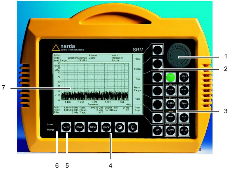
Fig. 6-1 Display and control elements
