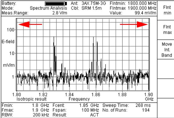
Fig. 8-27 Integrating the level value over a frequency band
