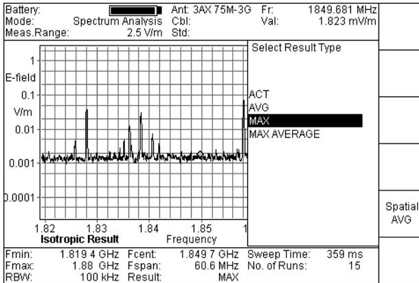
Fig. 12-14 The “Select Result Type” selection box and “Spatial AVG” softkey
