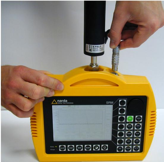
Fig. 5-3 Connecting the multi pin connectors
