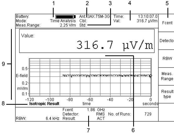
Fig. 10-2 "Time Analysis" mode measurement menu
