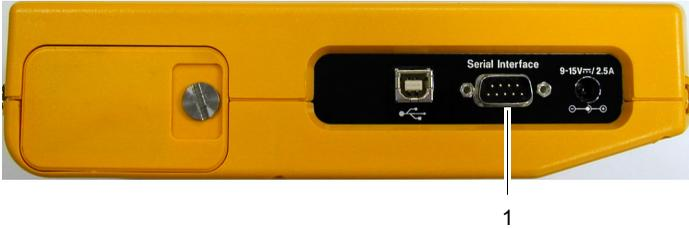
Fig. 17-1 Serial (1) and USB (2) interfaces
