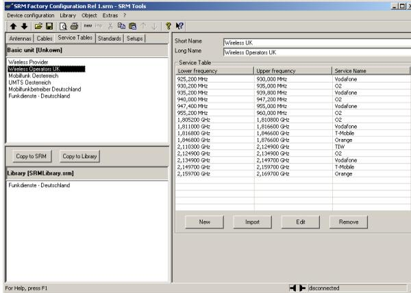
Fig. 16-8 "SRM-Tools" software in "Configuration" mode
