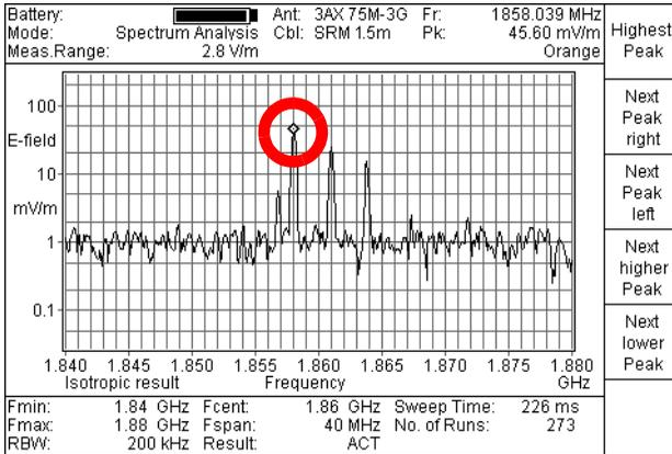
Fig. 8-21 Moving the marker with the **Highest Peak** softkey
