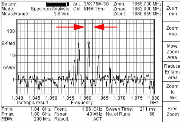
Fig. 8-18 Positioning the marker in the center of the zoom area
