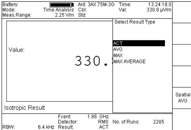
Fig. 12-15 The “Select Result Type” selection box and “Spatial AVG” softkey
