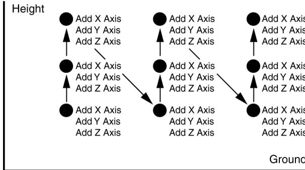
Fig. 12-3 Three separate measurements are needed at each point if a single axis antenna is used
