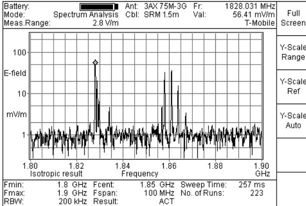
Fig. 8-9 Softkeys for selecting the display mode and scaling
