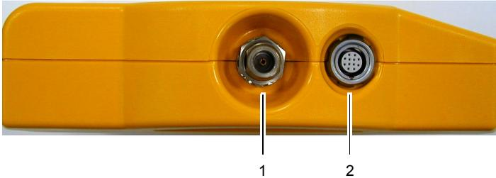
Fig. 6-3 Antenna and control cable connector sockets
