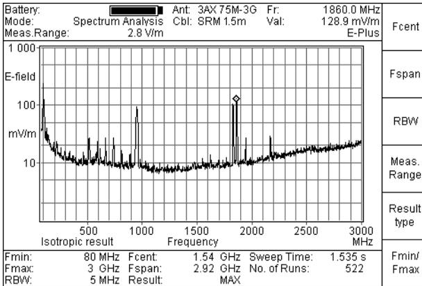
Fig. 11-1 “Spectrum Analysis” mode (Isotropic result)
