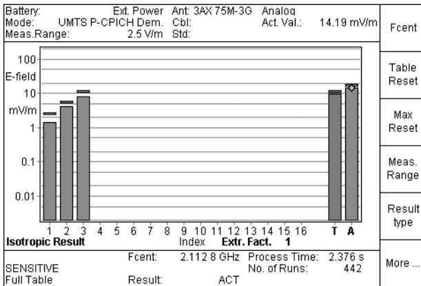
Fig. 9-5 Bar Graph display mode
