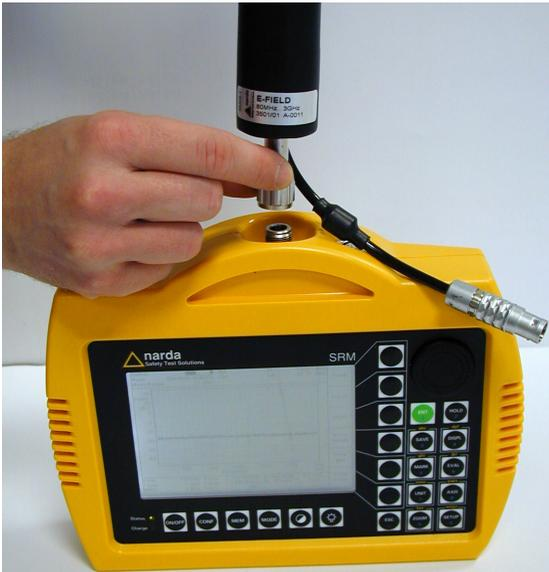
Fig. 5-2 Connecting up the N connectors
