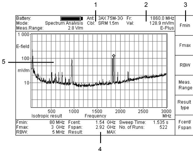
Fig. 6-2 LCD panel in "Spectrum Analysis" mode (example)
