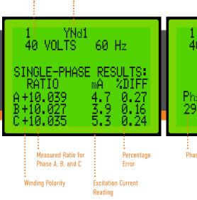
Test Voltage Transformer Type
