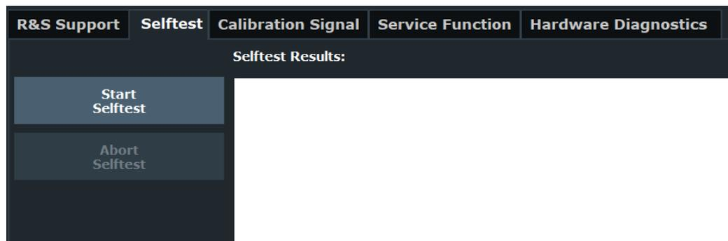
Once the self-test is started, all modules are checked consecutively and the test result is displayed. You can abort a running test.
