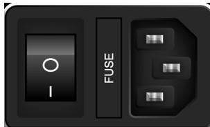
1. **WARNING!** The fuse is part of the main power supply. Handling the fuse while the power is on can lead to electric shock.
