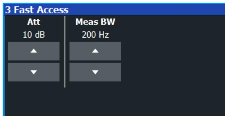
The advantage of the fast access panel is that it is easier and faster to change various settings in a single panel without having to find and access dialog boxes or softkey menus first. In addition, you can still view results while changing parameters, without dialog boxes blocking the view.
