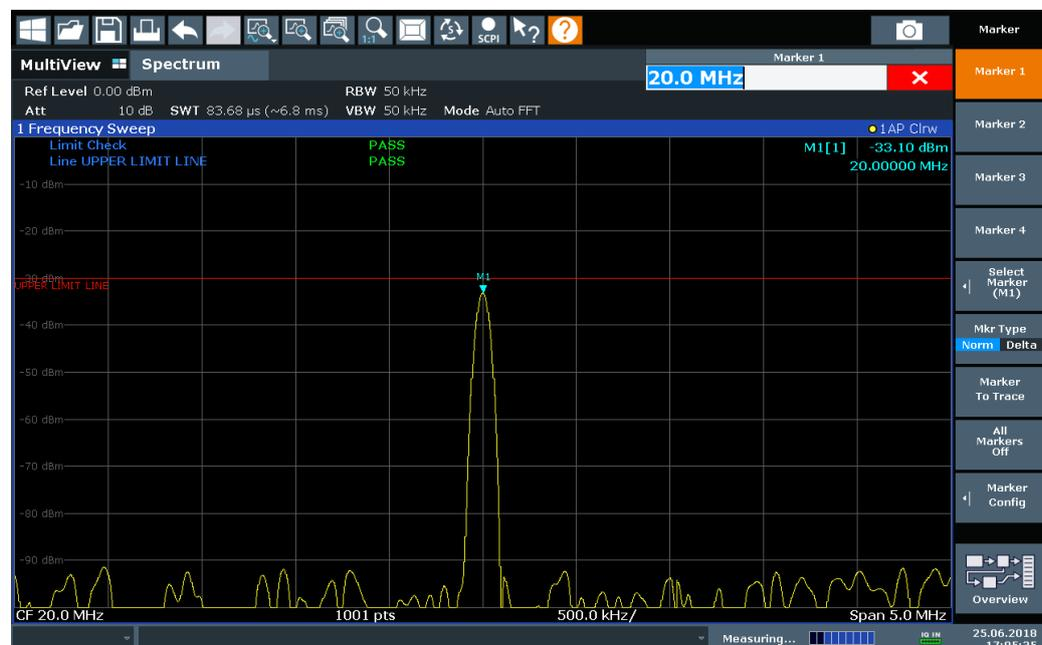
Figure 11-9: Example for an upper limit line
