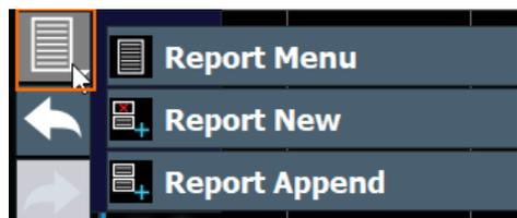
The R&S EPL1000 features a test report generator. A test report is a document that summarizes the results and configuration of measurements.
