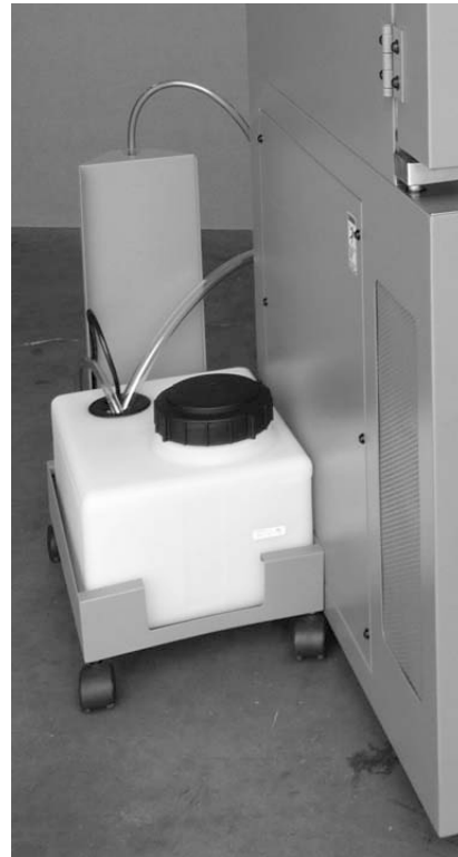
Finger-tighten the Water Supply and Drain connections to chamber. Plug pump wire into receptacle, turn clockwise to lock. Drain tube must not be submerged in the water. Installation behind chamber is not recommended because it may block the air vents.
