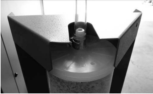
Use clamp on each end of filter to prevent leaking. Do not overtighten.
